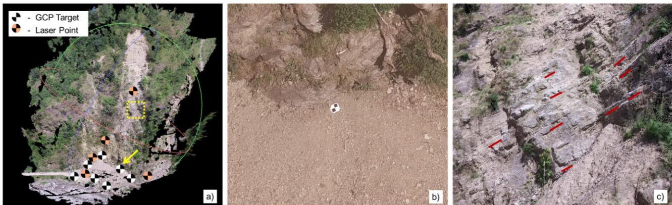
Figure 9. (a) Overview of co-seismic landslide east of Kathmandu with distributed ground control points and laser points used as check points; (b) view of target on the ground at location shown by arrow in (a); (c) landslide back-scarp illustrating foliation of the rock; red lines indicate locations where foliation orientation was interpreted from the 3D model.
