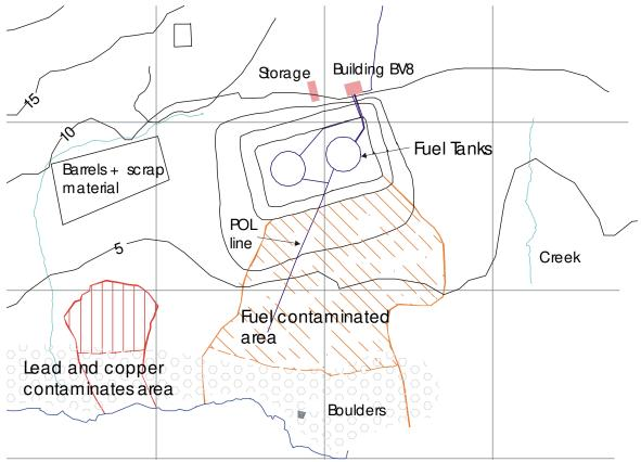
Figure 3. Plan view of fuel contaminated area.
