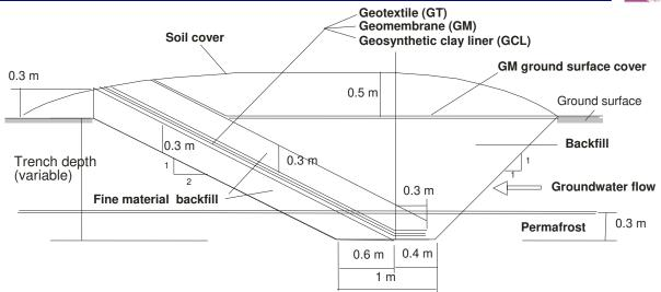
Figure 6. Installation of geosynthetic barrier system anchored in permafrost (Case 1).
