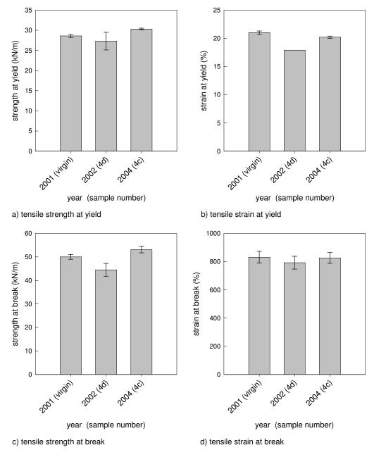
Figure 15. Mechanical load-strain properties of virgin and exhumed 1.5 mm-thick fluorinated HDPE geomembrane samples. Notes: 5 specimens per sample; error bars represent ±1 standard deviation.
