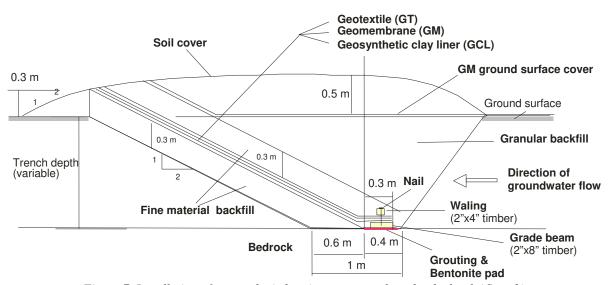
Figure 7. Installation of geosynthetic barrier system anchored to bedrock (Case 2).
