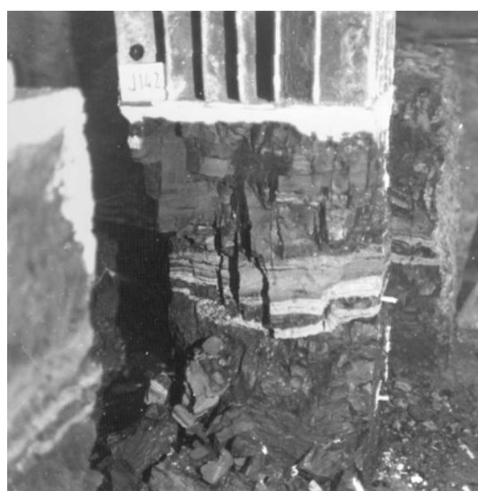
Figure 9. Failed block of coal after testing (Hudek, 1986).
