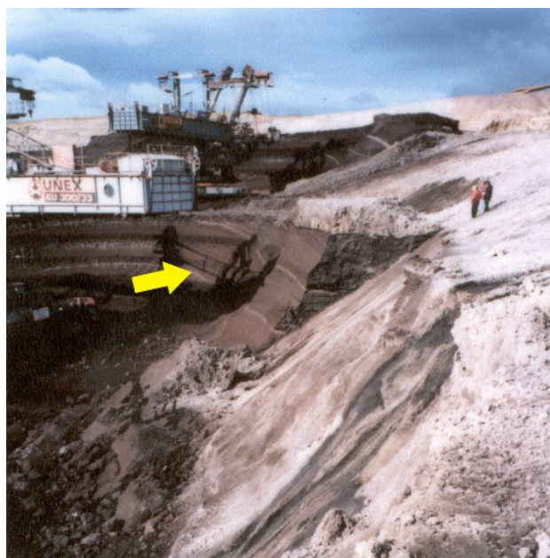
Figure 5. Jiri Mine - view of the 50 m thick coal seam (Vobornikova, 2000).
