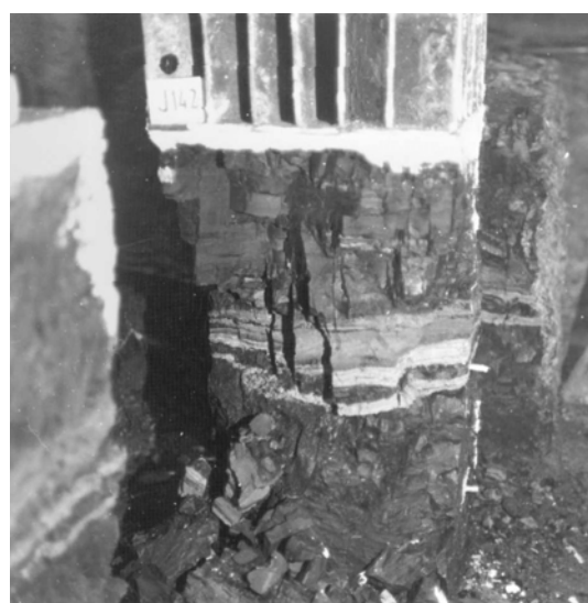
Figure 9. Failed block of coal after testing (Hudek, 1986).
