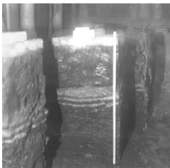
Figure 8. Blocks of coal prepared for in situ triaxial compression tests (Hudek, 1986).
