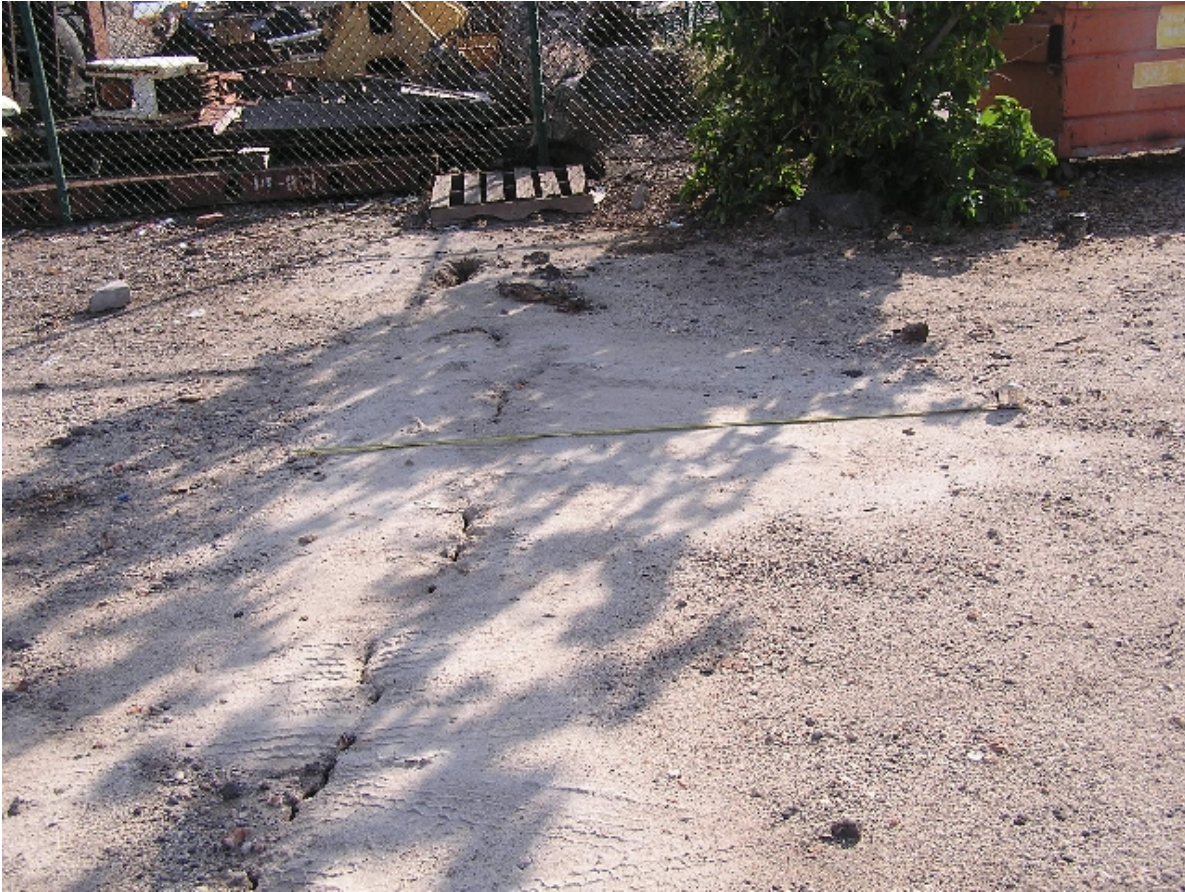
Figure 39. Location 27, Kawaihae Small Boat Harbor parking lot, adjacent boat yard at south side. Liquefied (white) sand was ejected from wide ground crack during the earthquake shaking.
