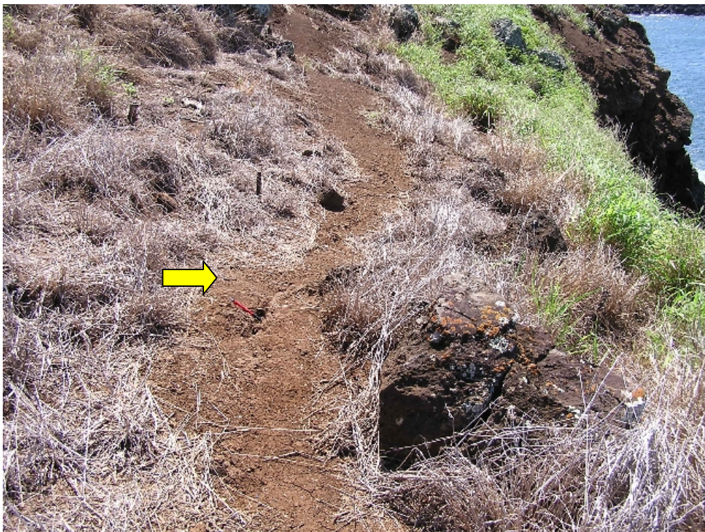
Figure 35. Location 23, Ala Kuakini Trail. Tension cracks behind cliff top (arrowed) in foreground.
