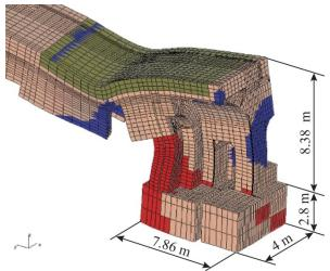
Figure 13. Deformation scheme (scale of deformations enlarged 500 times) and limit state areas in brickwork (defined by Mohr-Coulomb criteria) accounting for subsoil ground wash-out and decomposed timber piles. Shaded sections denote limit state areas generated by compressive and tensile stresses.
