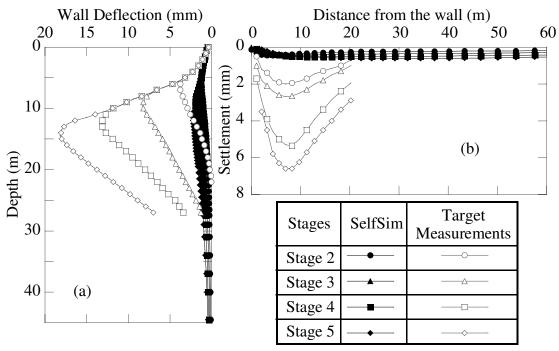
Figure 16. Computed deformations in Cluster 1 prior to SelfSim learning; a) wall deformations, and b) surface settlements, Shanghai excavation.
