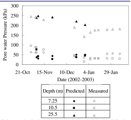
Figure 18. Comparison of predicted and measured pore water pressures for PA1 in cluster 1, Shanghai excavation.
