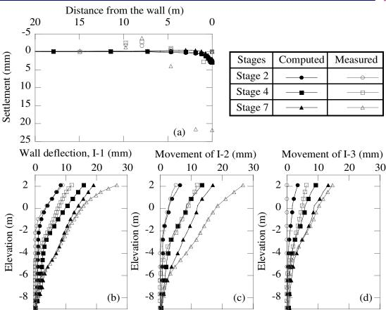
Figure 7. Computed response, two anchor section, Texas A& M excavation, after six passes of SelfSim learning with wall deformations (I-1), lateral movements of inclinometer I-3, and tieback loads.
