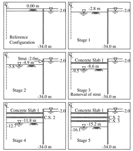
Figure 25. Excavation sequence in TNEC excavation in Taipei.
