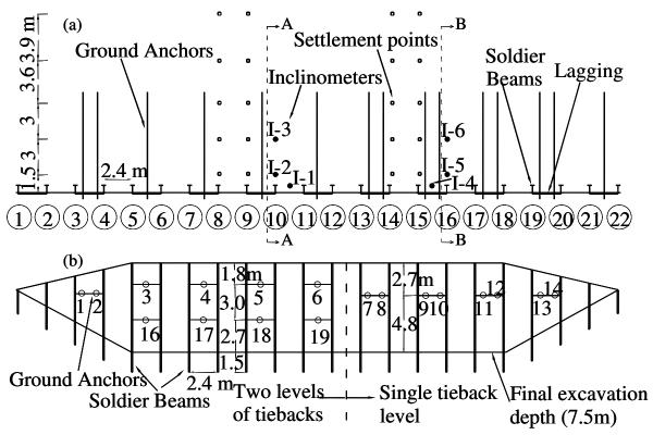
Figure 3. Schematic of Texas A&M University full scale model excavation site showing a) plan view and instrument locations, b) elevation view of the wall, inclinometer labels introduced in this study, modified after Weatherby et al. (1998).
