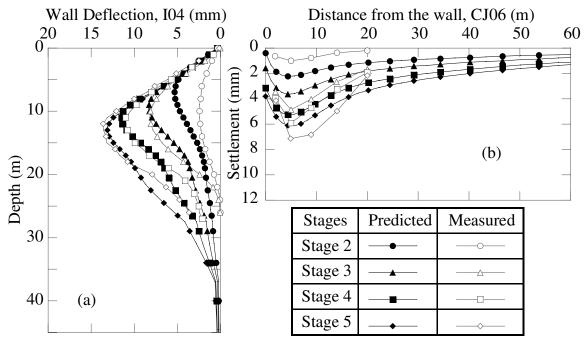
Figure 21. Predicted deformations in cluster 3 after six passes of SelfSim learning with cluster 1 deformations; a) wall deformations (104) and b) surface settlement CJ06, (middle slab was used), Shanghai excavation.
