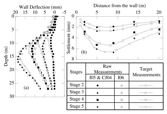
Figure 15. Original and target measurements for inverse analysis for a) lateral wall deflections of 105 & 106, and b) surface settlements CJ04, Shanghai excavation.
