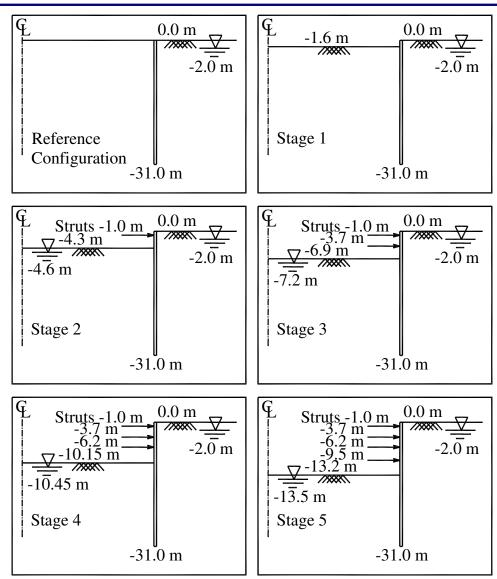
Figure 28. Construction sequence of Formosa excavation.
