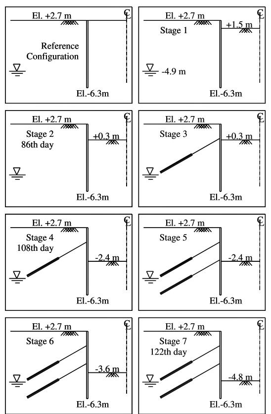
Figure 5. Construction sequence for two level tieback section of the Texas A&M University full scale model wall.
