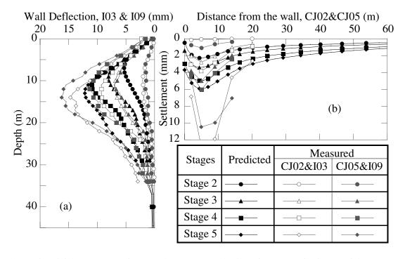
Figure 19. Predicted deformations in cluster 2 after six passes of SelfSim learning with Cluster 1 deformations; a) wall deformations (103 and 109) and b) surface settlement CJ02 and CJ05, (middle slab was used), Shanghai excavation.
