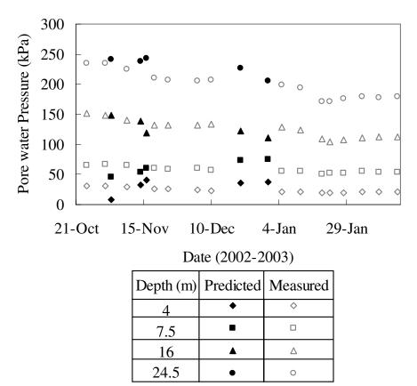
Figure 20. Comparison of predicted and measured pore water pressures for PA2 in cluster 2, Shanghai excavation.
