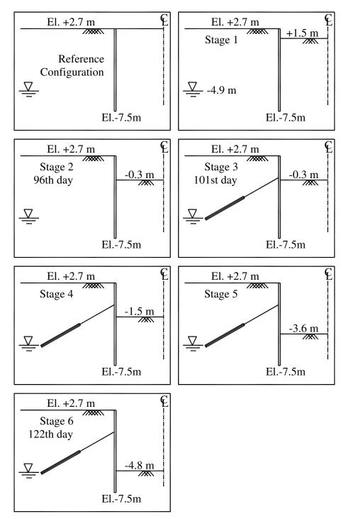
Figure 9. Construction sequence for single tieback section of the wall, Texas A& M excavation.
