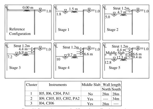
Figure 14. Construction sequence for different clusters, Shanghai excavation.
