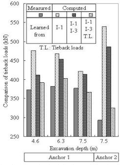
Figure 8. Comparison of measured and computed tieback loads in two-level tieback section of the wall, Texas A&M excavation.
