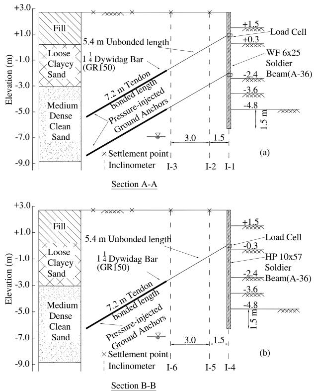
Figure 4. Sections of the Texas A&M University full scale model wall: a) two-level tieback, b) one-level tieback, modified after Weatherby et al. (1998).
