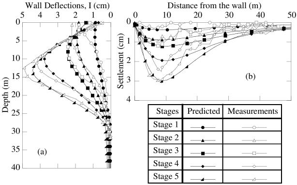
Figure 30. Predicted and measured excavation response for a) lateral wall deflections, b) surface settlements in Formosa excavation.
