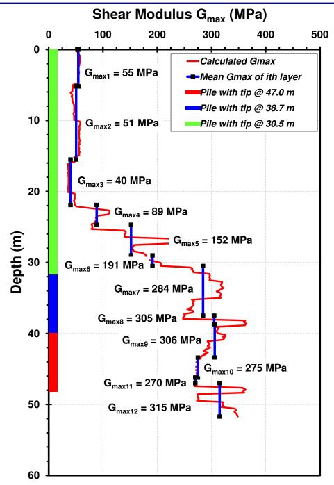
Figure 6. Profile of Small Strain Shear Modulus, G<sub>max</sub> for soil layers at EURIPIDES test site.
