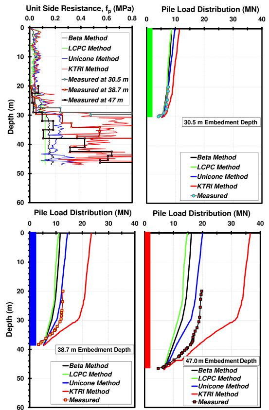
Figure 8. Unit side resistance and pile load distributions at 30.5 m, 38.7 m and 47.0 m embedment depths.
