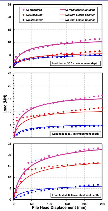
Figure 10. Load-displacement response for pile tests at location 1 EURIPIDES (measured and evaluated).
