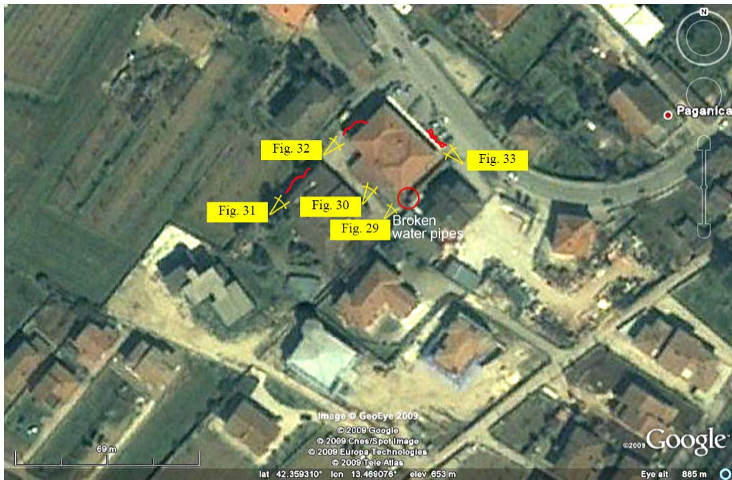
Figure 28. Plan view of Paganica site with marked positions of ground fissures, paved walkway cracks and broken water pipes. Directions of photo shots are indicated by yellow signs.
