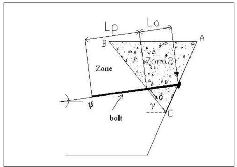
Figure 14. Scheme of interaction between rock mass and bolt; La: length of bolt in unstable zone (zone 1); Lp: length of bolt in stable zone (zone 2);  $\delta$ : block displacement along sliding;  $\psi$ : dip of bolt from horizontal plane;  $\gamma$ : angle between sliding direction and horizontal plane.
