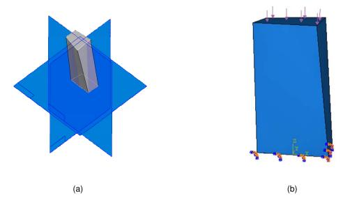
Figure 11. (a) View of pillar No. 23 (see Figure 7) as modeled with ABAQUS software (Hibbit, Karlsson and Sorensen, Inc., 1994); (b) different 3D view of same pillar with boundary conditions and applied loads.
