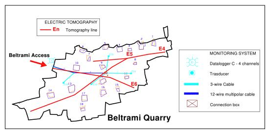
Figure 6. Map of Beltrami quarry showing roofs of pillars(blue) and base (green), monitoring system and tomography lines.
