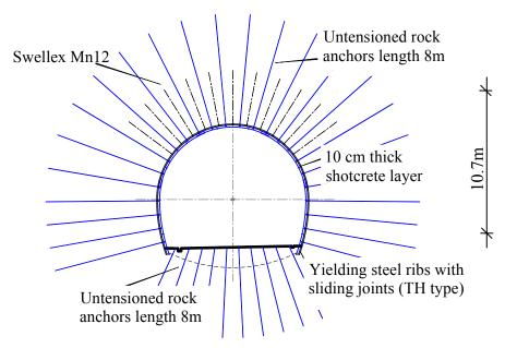
Figure 6. Tunnel cross section showing the excavation-support system P7.3 adopted between chainage 1267 and 1324 m. For sake of simplicity the face pre-reinforcement is not shown.
