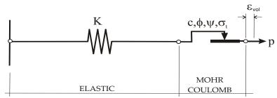
Figure 20(a). CVISC model: volumetric behaviour.
