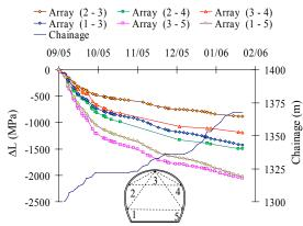
Figure 11. Convergences of section 1297m versus face advancement.
