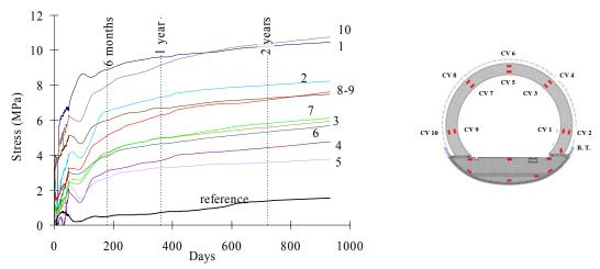
Figure 18. Stresses in final lining at chainage 1457 m.
