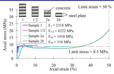
Figure 10. Characteristic stress-strain diagram of a HiDCon element.
