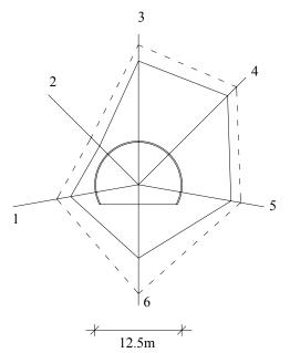
Figure 15. Multi-position borehole extensometers at chainage 1443 m: 1% strain at the end of stage 1 (dashed line) and before the installation of final lining (solid line).
