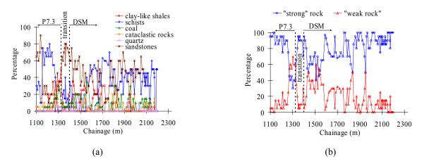
Figure 4. Percent distribution of (a) rock typesand (b) "strong" (sandstones and schists) and "weak" (coal and clay-like shales) rocks at the face.
