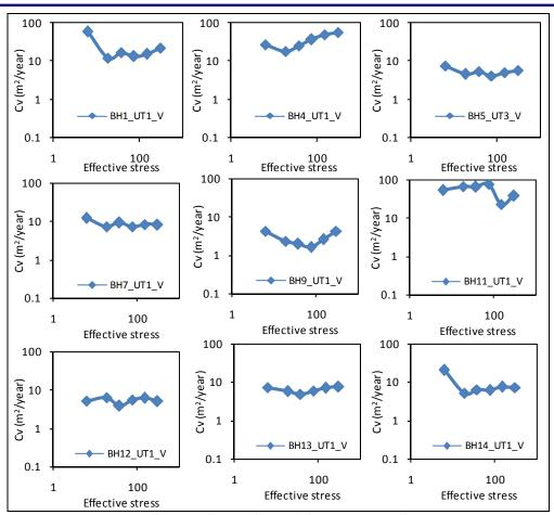
Figure 7. Coefficients of vertical consolidation against effective stresses.
