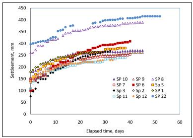
Figure 13. Ground settlements with time.
