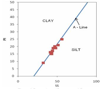
Figure 4. Data points with respect to A-line.
