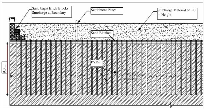
Figure 12. Detail of the ground improvement works (schematic).
