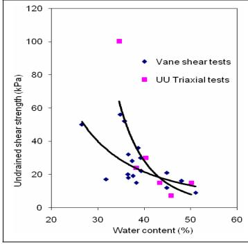
Figure 5. Undrained shear strength versus water content.
