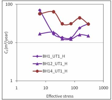
Figure 8. Coefficients of horizontal consolidation versus effective stresses.
