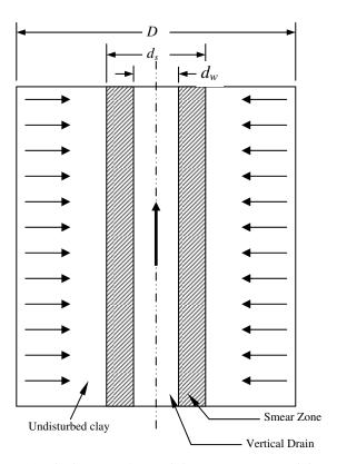
Figure 10. Idealization of consolidation using vertical drain.
