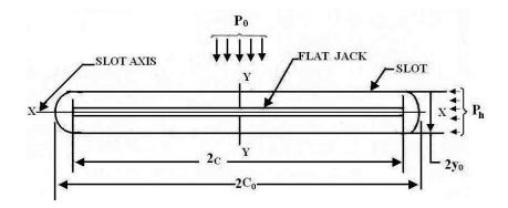
Figure 5. Stress field around the slot.
