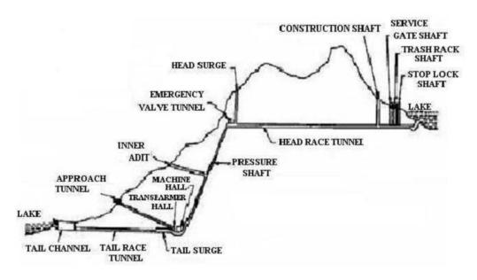
Figure 2. Schematic layout of Koyna H.E.Project stage-IV.
