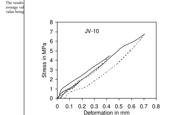
Figure 10. Stress deformation envelope of flat jack test location JV 10 in breecia in pilot shaft.
