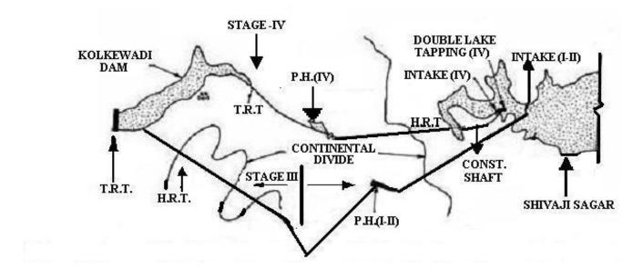
Figure 1. Koyna H.E. Project (Stage I-II-III-IV) schematic layout.
