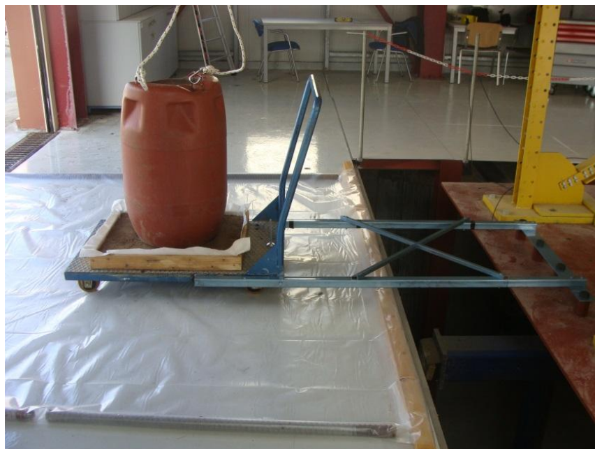
Figure 16. Mechanism used for performing shaking tests on the water filled plastic container by utilizing the University of Patras Shaking Table facility.
