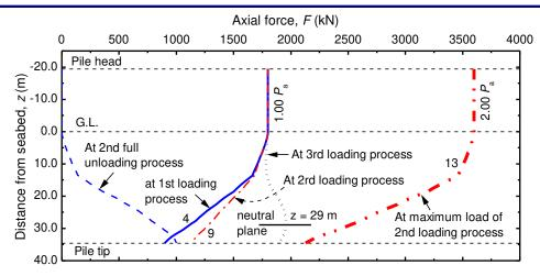
Figure 26. Calculated distributions with depth of the pile axial forces of the TSC1 at the BOR test.
