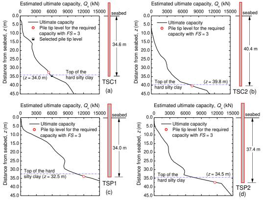
Figure 7. Estimated ultimate capacity with depth and selection of the pile tip level for:
