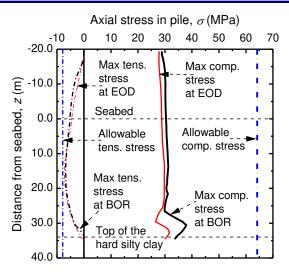
Figure 23. Distribution with depth of the maximum tensile and compressive stresses in the pile during driving of the TSC1.
