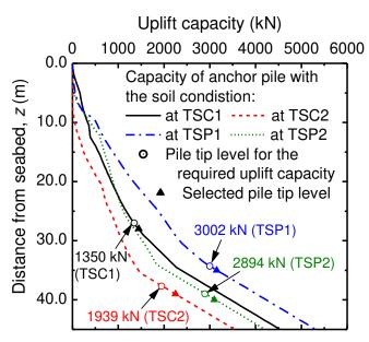
Figure 12. Uplift capacity of the anchor piles with the soil conditions at the TSC1, TSC2, TSP1 and TSP2.
