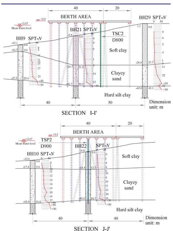
Figure 5. Geological sections at locations of the test piles: (a) TSC2. (b) TSP2.
