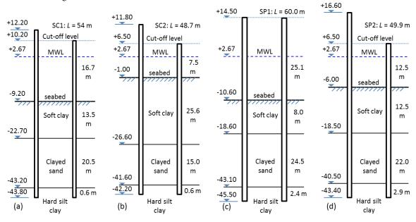
Figure 9. Illustration of the four test piles before and after cutting the pile to the cut-off level.
