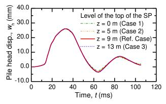
Figure 22. Calculated pile head displacement with different heights of the soil plug.
