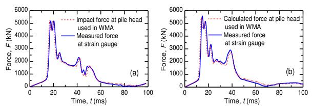
Figure 17. Calculated impact forces at the pile head, together with measured forces of the TSC1 at (a) EOD. (b) BOR.
