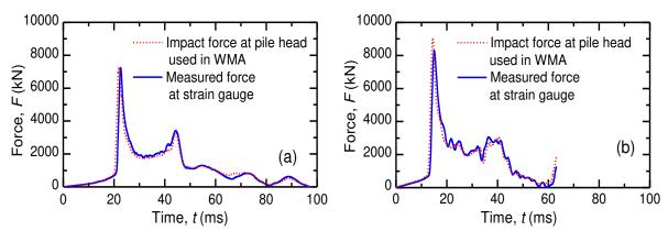
Figure 18. Calculated impact forces at the pile head, together with measured forces of the TSP1 at (a) EOD. (b) BOR.
