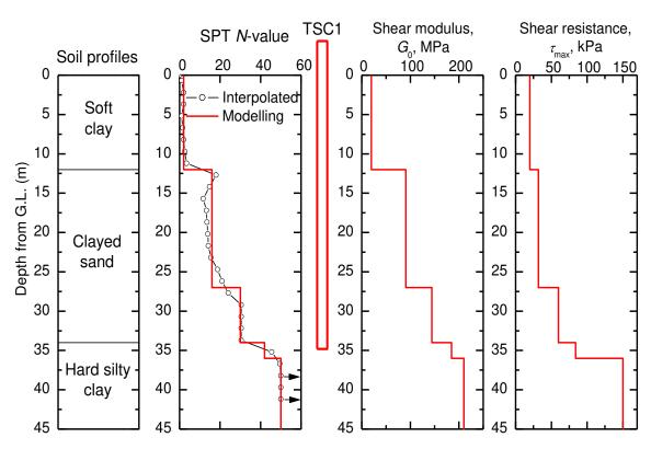
Figure 15. Modelling of the test ground at the test pile TSC1.
