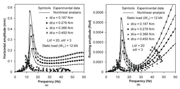
Figure 11. Comparison between the Response Curves obtained from Experiment and Continuum Approach of Han (1997)[(a) Horizontal And (b) Rocking Mode]
