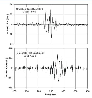
Figure 2. Variation of S-Wave Arrival with Time at Two Boreholes of Seismic Crosshole Tests.
