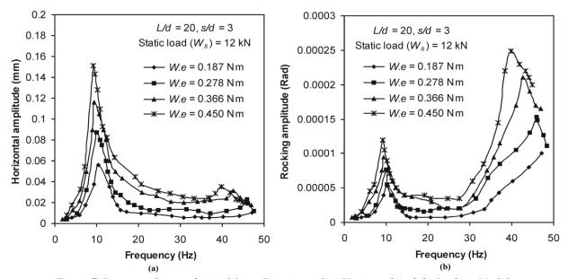
Figure 7. Response Curves obtained from Experiment [(a) Horizontal And (b) Rocking Mode].
