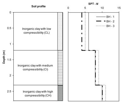
Figure 1. Soil Profiles and Uncorrected SPT-N Value With Depth.
