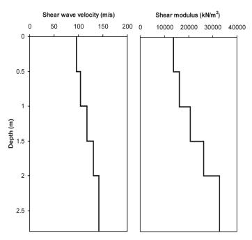
Figure 3. Variation of Shear Wave Velocity And Shear Modulus of Soil With Depth.
