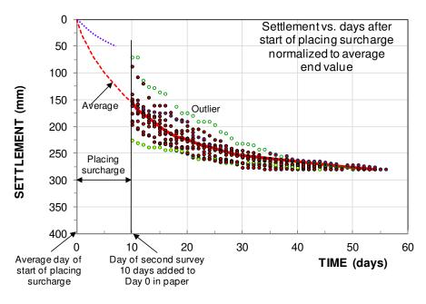
Figure 2. Settlement measured at the benchmarks normalized to the average end values.
