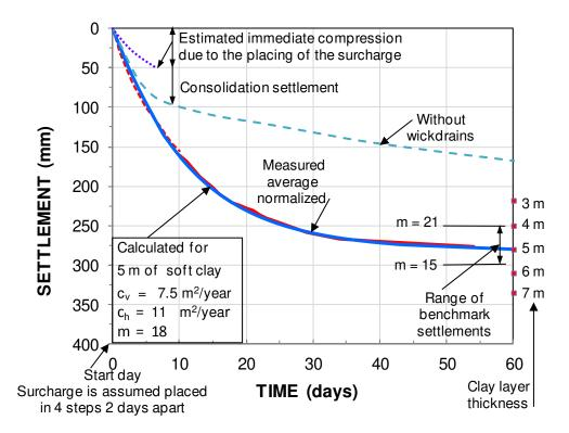
Figure 4. Average measured and calculated settlements.
