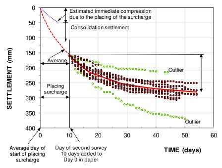
Figure 1. Settlement measured at the benchmarks shifted 10 days.
