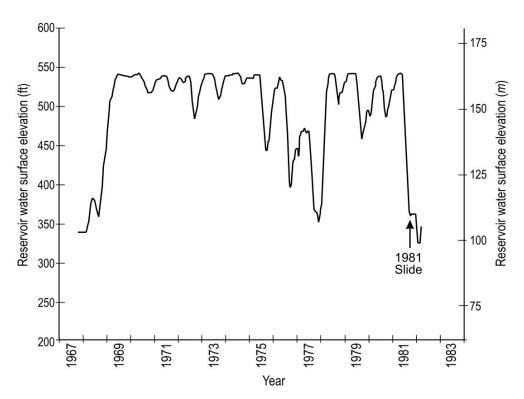
Figure 1. San Luis Dam site: (a) Elevation view of the 1981 slide; (b) Reservoir operational history.
