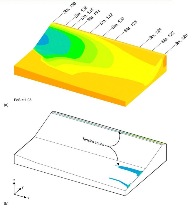
Figure 9. Slope stability analysis results of three-dimensional continuum model between stations 120 and 138.
