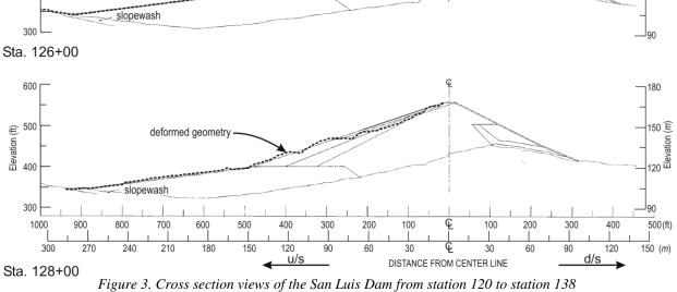
showing the original and deformed configuration of the dam.
