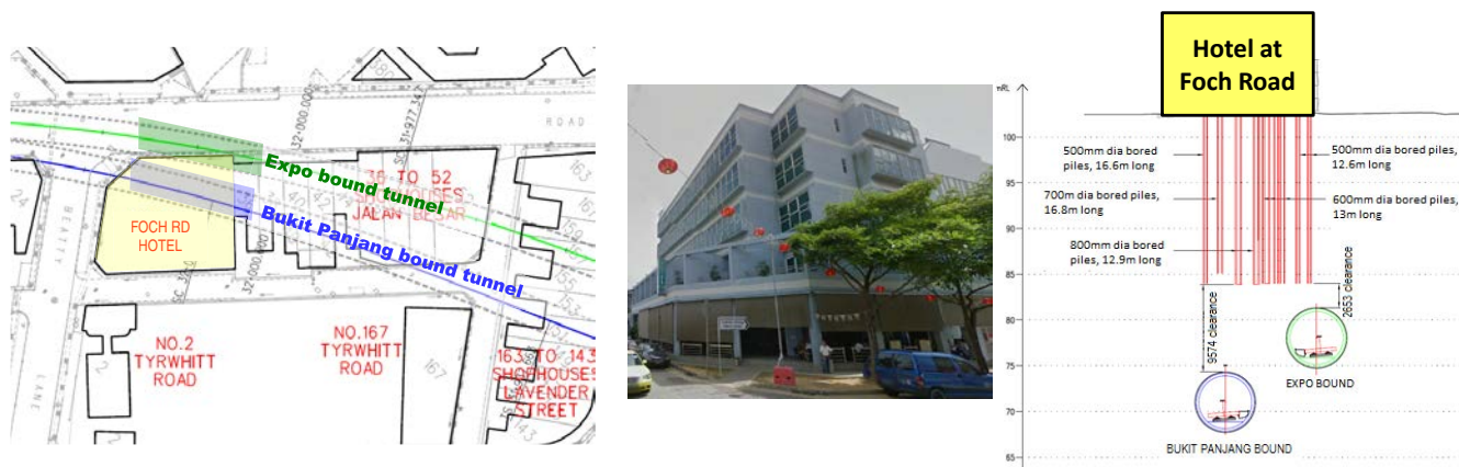
Figure 10. Location map and cross-sectional view of tunnelling directly below hotel at Foch Road.
