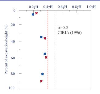
Figure 10. APD developed for Bukit Timah granite residual soils.
