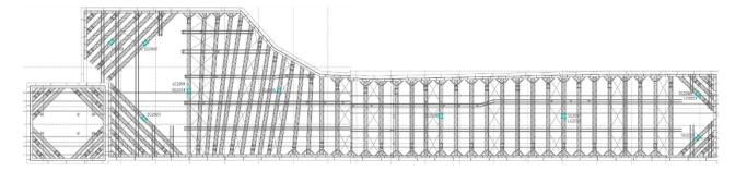
Figure 3. Typical strutting arrangement plan.
