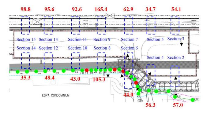
Figure 11. Effect of recharging on ground settlements.
