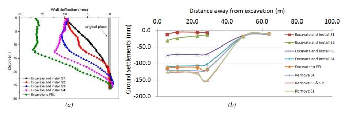
Figure 6. Lateral response for inclinometer I2509 and the ground settlement for section 9: (a) Lateral wall deflections; (b) Ground settlements.
