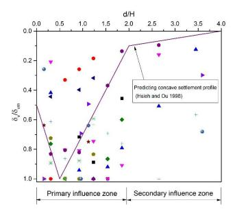
Figure 15. Comparison of ground settlement profiles against Concave settlement by Hiseh and Ou 1998.
