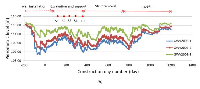
Figure 7. Piezometric level changes of: (a) GWV2005; and (b) GWV2006.
