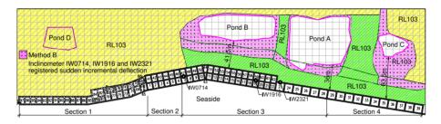
Figure 7. Stage 2 reclamation - Extent of reclamation where three inclinometers IW0714, IW1916 and IW2321 showed significant incremental deflection or sudden plunge (Method B :: ).
