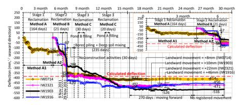
(b) Deflection of capping beam of seawall for section 3.
