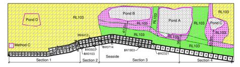
Figure 8. Stage 3 reclamation - Filling of ponds B, A, and C showed insignificant incremental deflection of the seawall (Method  $C \square$ ).
