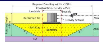
\* 150 m wide and 44 m deep sandkey is necessary to cut off the deep slip failure plane. (c) A safe sandkey solution but not buildable.
