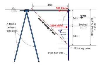
\* Not applicable to provide a horizontal pull back reaction in the A-frame and an adequate single row steel structural wall.
