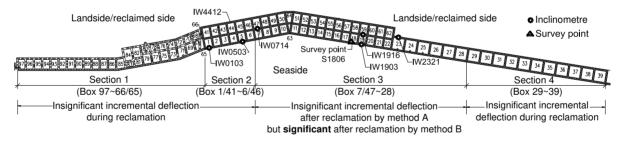
(c) Inclinometers at various sections of seawall.
