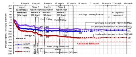
(a) Deflection of capping beam of seawall for section 2.
