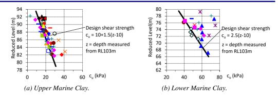
Figure 5. Undrained vane shear strength of soft clay. Note: Reduced level is the ground elevation level of the reclaimed fill.
