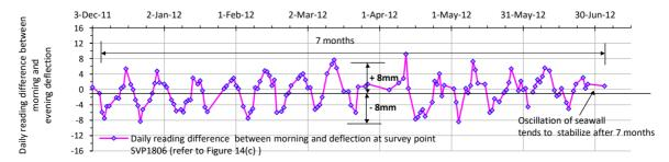
Figure 16. Difference in seawall deflection registered between morning and evening reading for survey point 1806.
