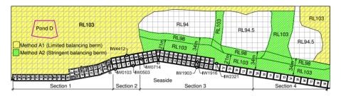
Figure 6. Stage 1 reclamation - Extent of reclamation where the seawall deflection was in accordance with the anticipated deflection (Method A1 & Method A2 ).
