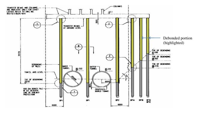
Figure 3. Schematic illustrating de-bonding length.
