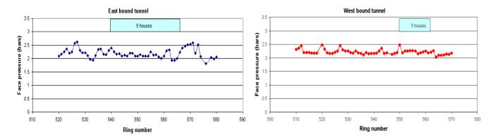
Figure 5 Application of face pressure.
