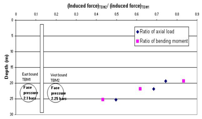
Figure 18. Effect of face pressure on pile response.
