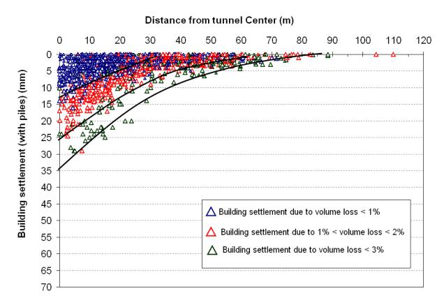
Figure 19. Tunnelling induced piled-building settlement.
