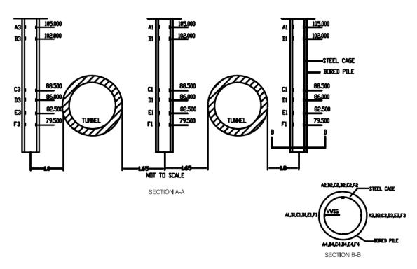
Figure 9. Six levels of strain gauges installed along the piles.
