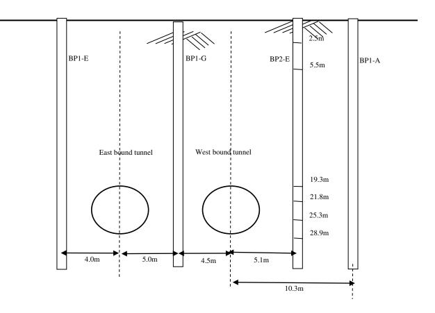
Figure 10. Illustration of pile positions relative to tunnels.
