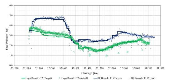
Figure 4. Face Pressure Plot for Tunnel 1 and Tunnel 2.
