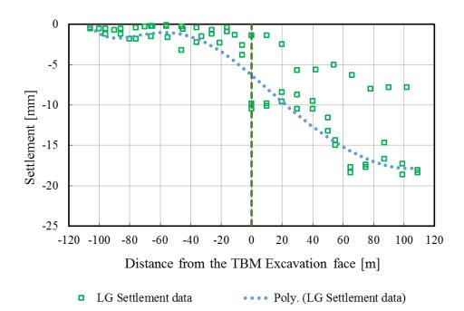
Figure 12. Surface settlement ahead of TBM excavation face.
