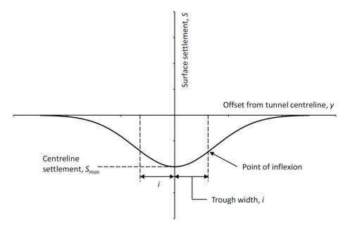
Figure 6. Ground settlement trough induced by a single tunnel.
