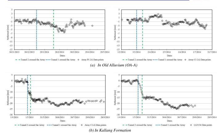
Figure 11. Maximum surface settlement over time recorded by various arrays.
