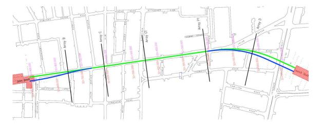
Figure 3. Location of monitoring instrumentation arrays along the alignment.
