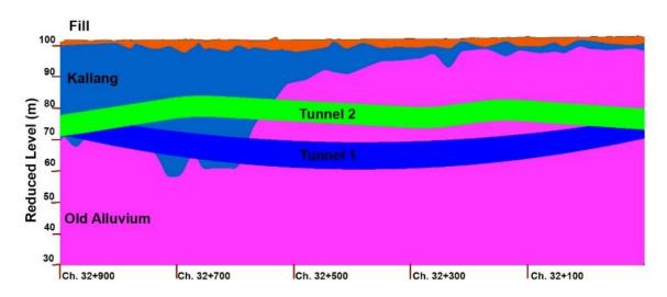
Figure 2. Geological profile along the alignment.
