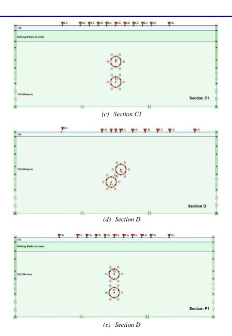
Figure 9. Ground information and array arrangement.
