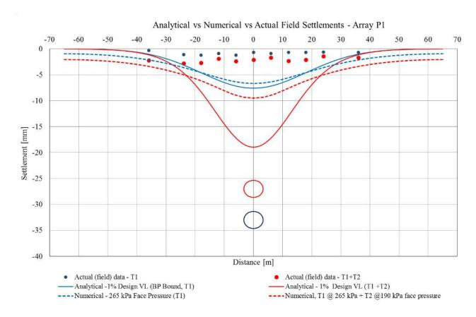
Figure 10. Comparison of Empirical results, numerical results and field measurements.
