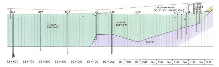
Figure 3. Geological longitudinal section of the embankment (Megalomastora 2012).
