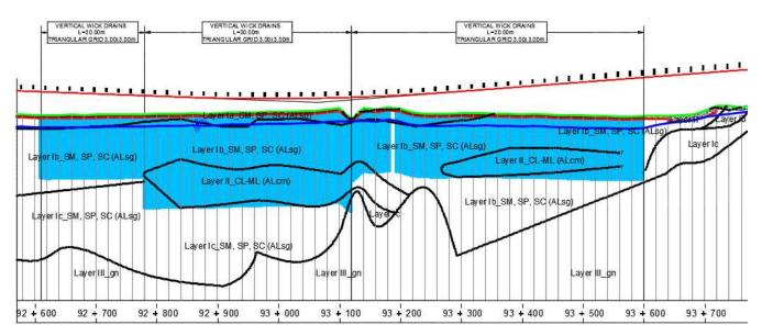
Figure 9. Longitudinal section of the embankment with the proposed installation of vertical drains.
