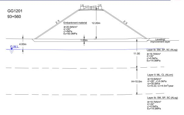
Figure 5. Critical cross-section used in the geotechnical calculations of the embankment.
