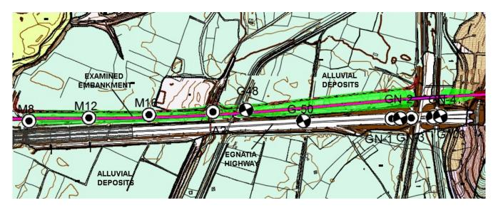
Figure 2. Geological plan view of the embankment with boreholes' locations (Megalomastora 2012).
