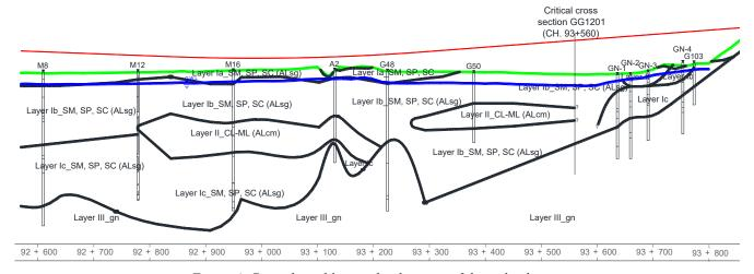
Figure 4. Geotechnical longitudinal section of the embankment.
