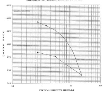
Figure 4. Typical 1D incremental oedometer lab test results from the CH soils at the site.
