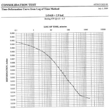
Figure 5. Typical log of time consolidation lab test results from the CH soils at the site.
