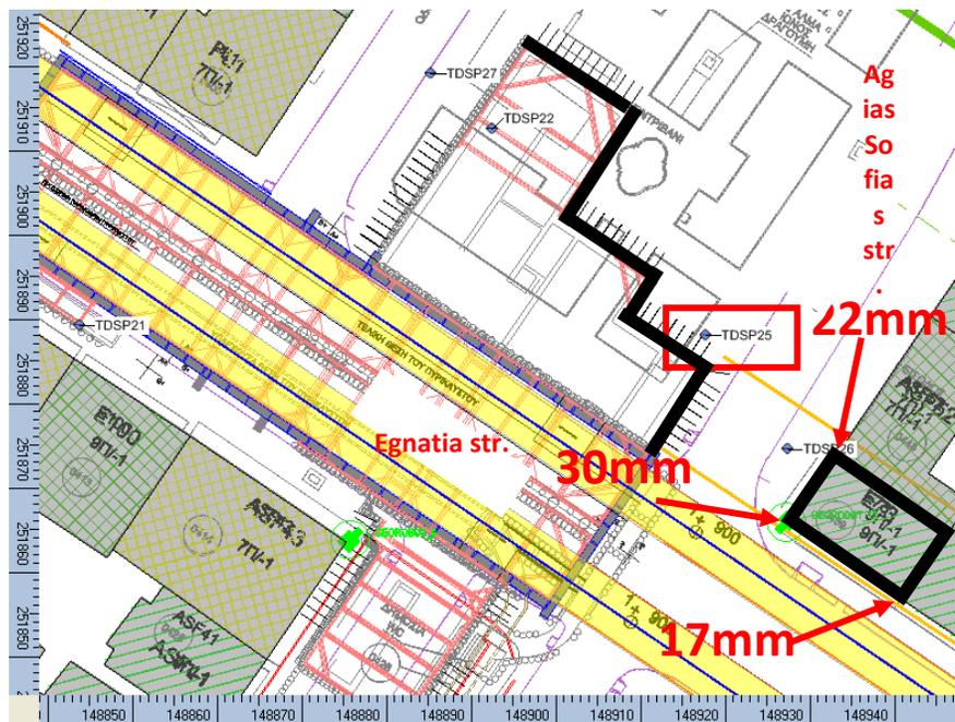
Figure 8. In situ measurements of vertical displacements .
