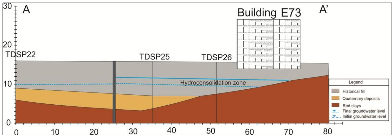
Figure 14. A-A' geological cross-section pointing the hydroconsolidation region.
