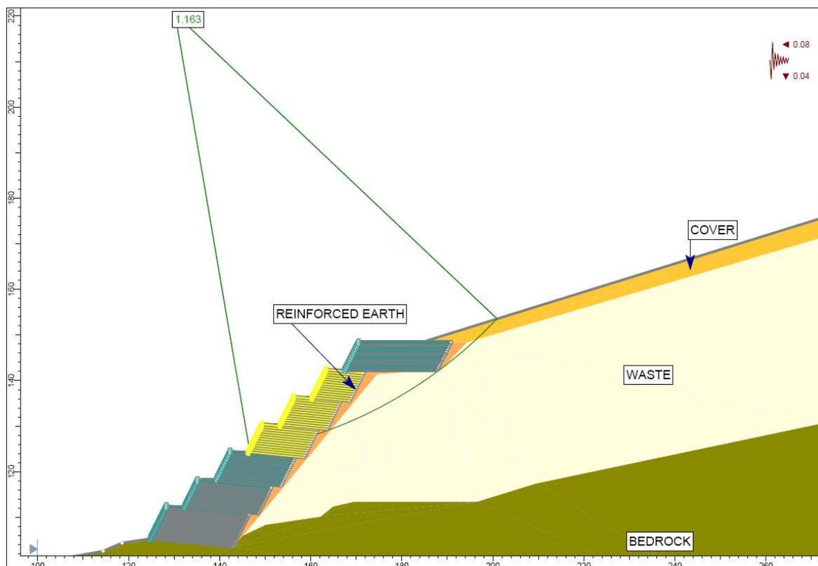
Figure 10. Global stability analysis results (seismic loading conditions).
