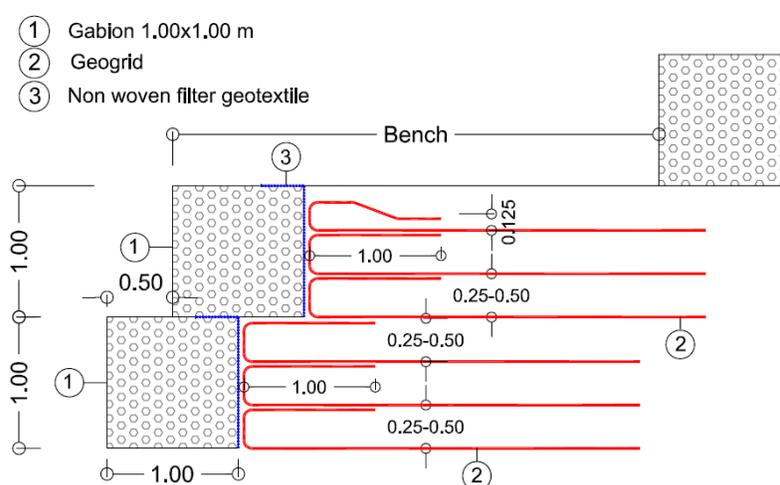
Figure 8. Reinforced earth gabion and geogrid details.
