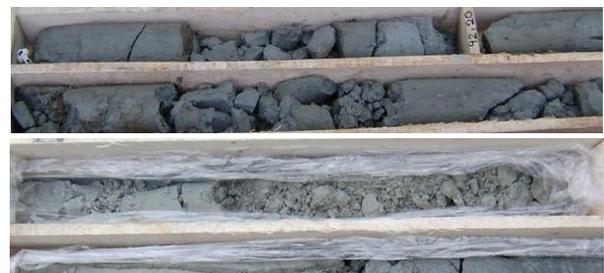
Figure 7. Typical core samples and engineering geology interpretation for the sandstone- siltstone units SS1 to SS4
