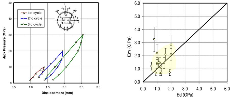
Figure 13. Typical Example of Dilatometer test results on the sandstone unit (left) and a comparison of the rock mass moduli (right) measured directly by dilatometer testing ( $E_d$ ) and estimated indirectly through the Hoek and Diederichs (2006) empirical relation ( $E_m$ ).
