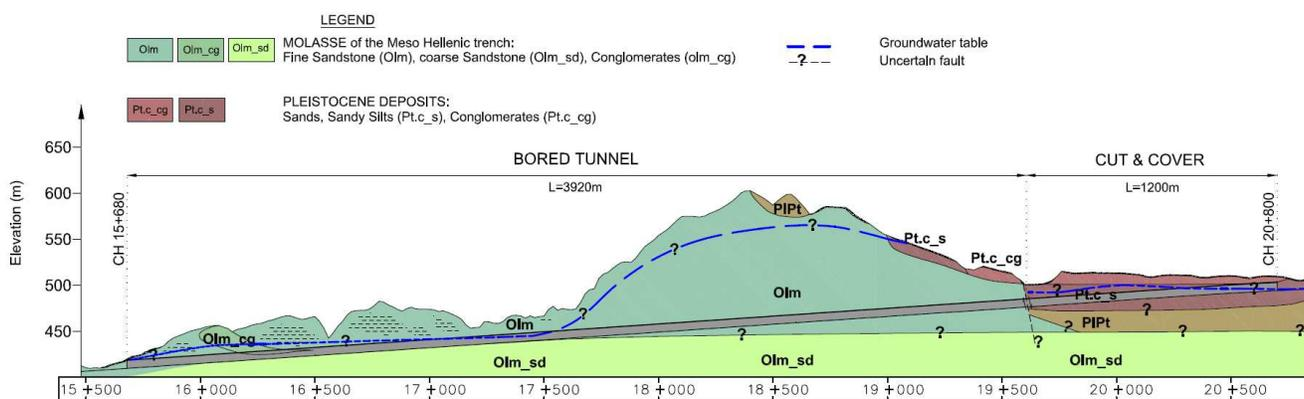
Figure 4. Tunnel Geological profile. Vertical exaggeration 4:1.
