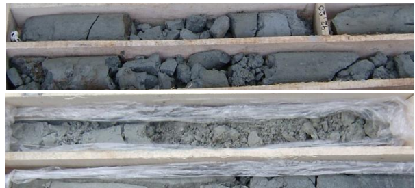
Figure 7. Typical core samples and engineering geology interpretation for the sandstone- siltstone units SS1 to SS4 (Note: RMT: Rock Mass Type).
