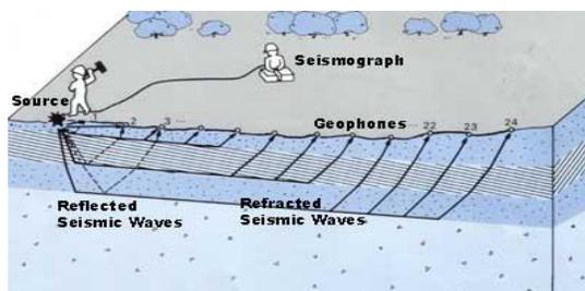
Figure 4. Typical set up for seismic refraction survey.
