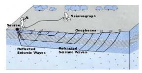
Figure 4. Typical set up for seismic refraction survey.
