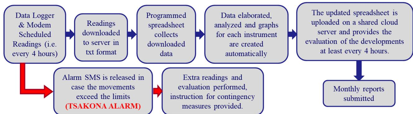
Figure 17. Automated monitoring procedure – Flow chart.
