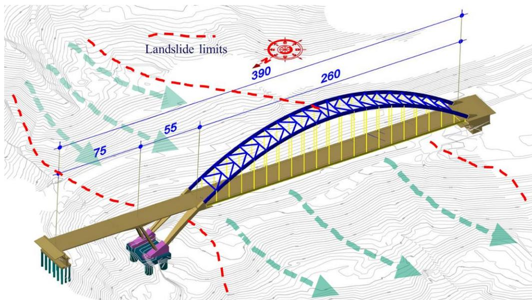
Figure 2. The Tsakona Bridge overpassing the active landslide.
