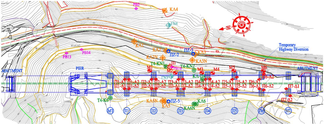
Figure 15. Arrangement of the geotechnical instruments in plan-view.
