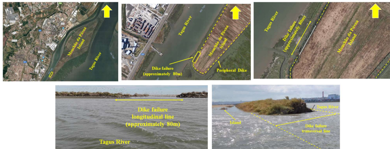
Figure 38. Location and view of the dike failure.
