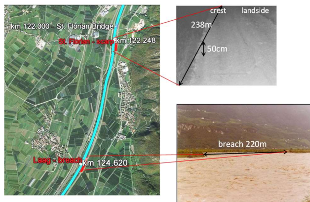
Figure 16. Overview of the two considered segments of the Adige River at Laag and St Florian
