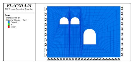
Figure 6. Initial sumulation of the model and the boundary condition.
