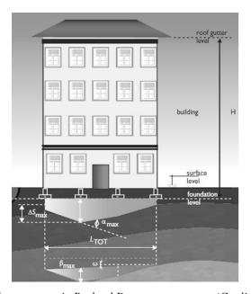
Figure 19. Related parameters in Burland Damage assessment (Guglielmetti et al. 2008).
