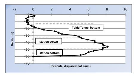
Figure 18. Horizontal displacement in section CC - left side of the station (based on numerical modeling).
