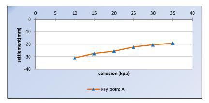
Figure 14. Effect of cohesion C on the surface settlement (for point A in Figure 9).
