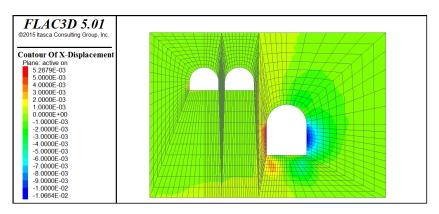
Figure 10. Horizontal displacement in soil mass after station excavation.
