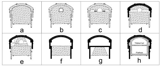
Figure 4. Schematic stages of the station construction.
