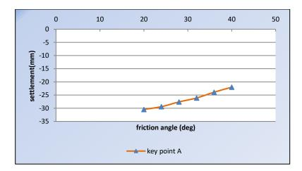
Figure 13. Effect of  $\varphi$  (friction angle) on the surface settlement (for point A in Figure 9).
