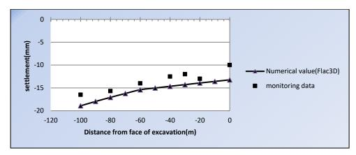
Figure 12. Monitoring & numerical results in longitudinal axis (for section ZZ in Figure 9).
