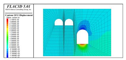
Figure 11. Vertical displacement in soil mass after station excavation
