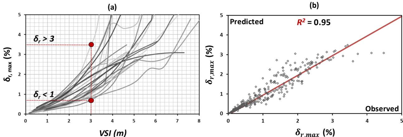
Figure 3. (a) Correlation of  $\delta_{r,max}$  as obtained from the FE analysis with VSI; and (b) observed (FE analysis) vs. predicted using the proposed nonlinear regression model equation maximum drift ratio  $\delta_{r,max}$ .
