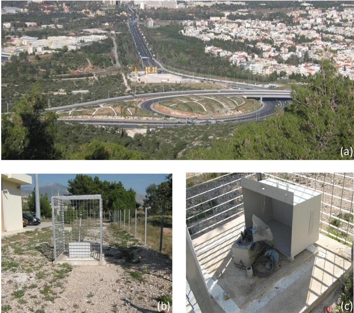
Figure 17. View of one accelerograph station. (a) The highway section monitored; (b) The station with the GPS antenna; (c) Close-up of Recording Instruments and wiring.
