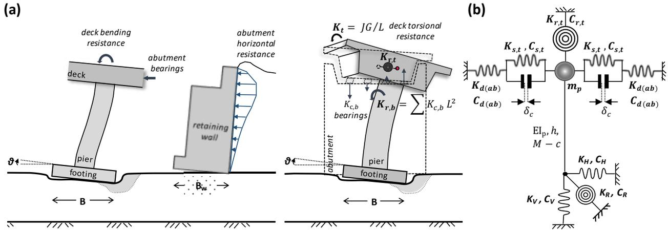
Figure 5. Simplified model accounting for key structural components, nonlinear SSI, and abutment stoppers of clearance  $\delta_c$ : (a) schematic illustration of key mechanisms; and (b) outline of the model.
