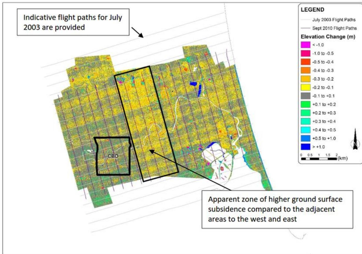
Figure 3. Banding related to LiDAR flight paths, T+T (2015).
