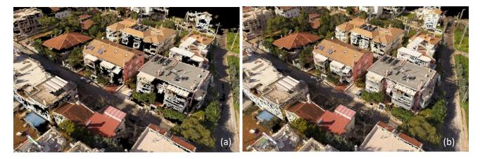
Figure 13. Comparison of point cloud data generated with (a) single pass and camera orientation pointing downwards only and (b) with double pass and camera orientation pointing downwards and obliquely. Notice the difference in the detail of the facades of the buildings, which is better captured by the oblique camera orientation.
