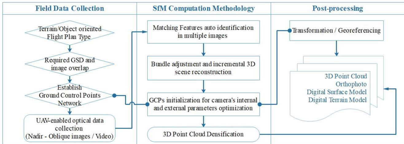
Figure 1. Schematic of the UAV-enabled SfM process.
