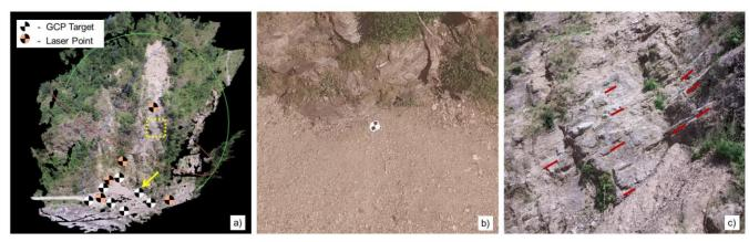
Figure 9. (a) Overview of co-seismic landslide east of Kathmandu with distributed ground control points and laser points used as check points; (b) view of target on the ground at location shown by arrow in (a); (c) landslide back-scarp illustrating foliation of the rock; red lines indicate locations were foliation orientation was interpreted from the 3D model.
