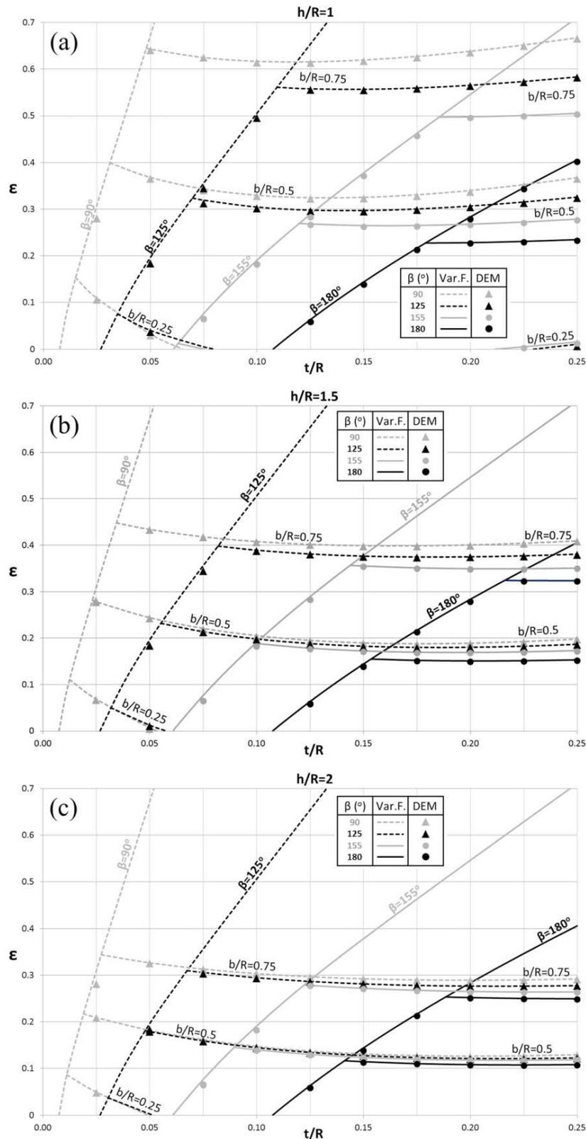
Figure 7. Seismic coefficient  $\epsilon$  for different geometries of the single-nave barrel vault with buttresses that are allowed to develop horizontal ruptures. Lines: Results from the variational formulation. Isolated symbols: Results from the Discrete Element Method (DEM).
