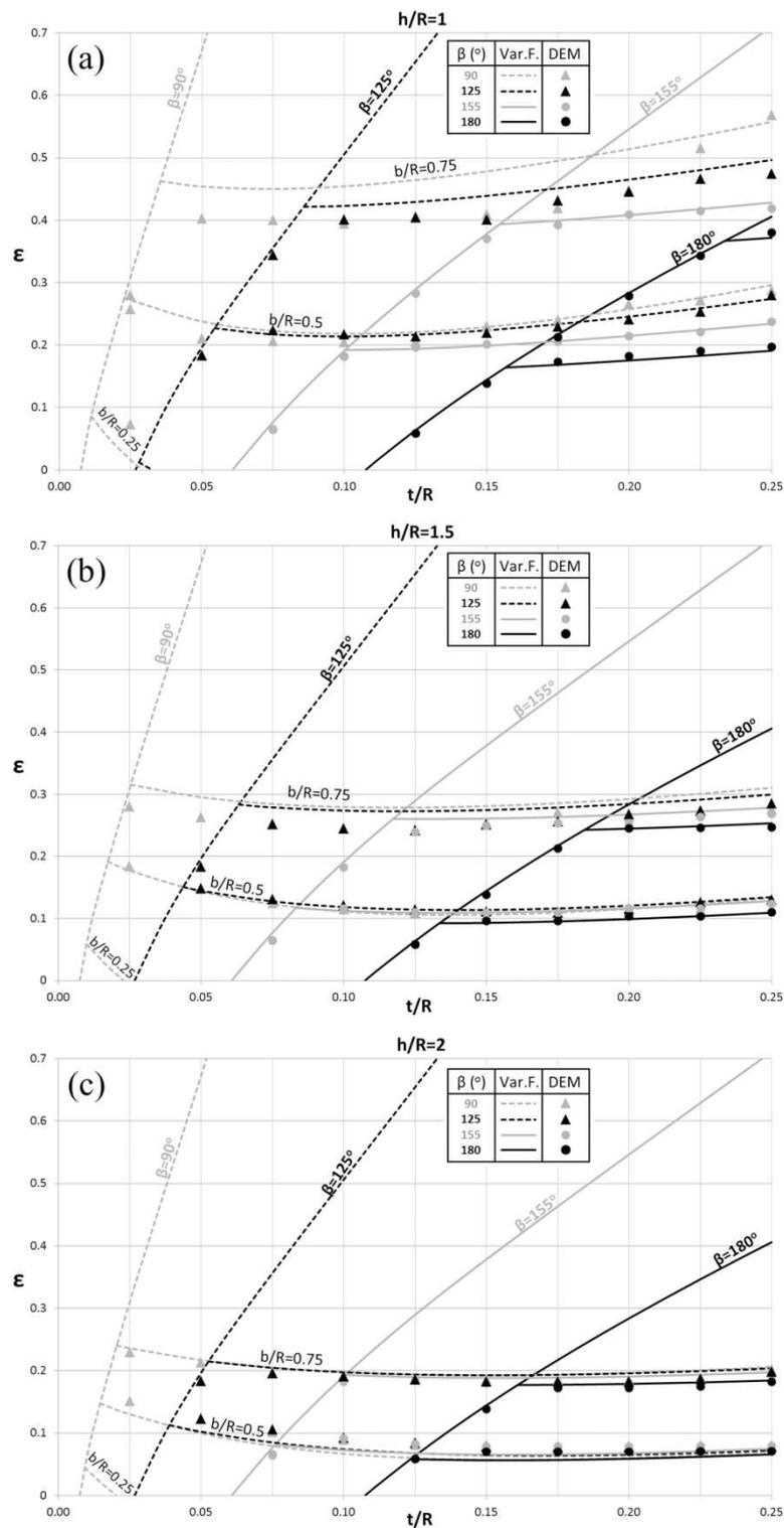
Figure 10. Seismic coefficient  $\epsilon$  for different geometries of the single-nave barrel vault with buttresses that are allowed to develop an oblique elongation failure. Lines: Results from the variational formulation. Isolated symbols: Results from the Discrete Element Method (DEM).
