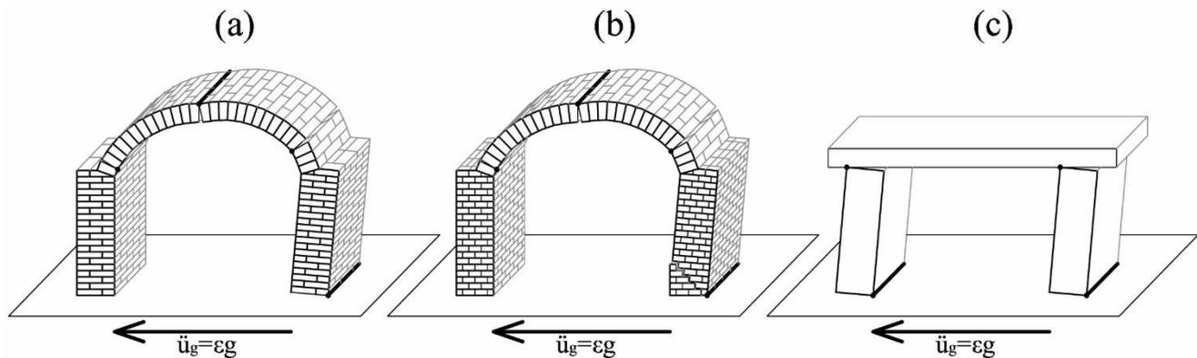
Figure 1. Single nave barrel vault subjected to a horizontal ground acceleration,  $\ddot{u}_g = \varepsilon g$ . (a) Horizontal rupture at the base of the buttress, (b) oblique rupture, (c) the rocking frame.
