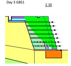
Figure 16. Critical slip surface slope stability analysis.
