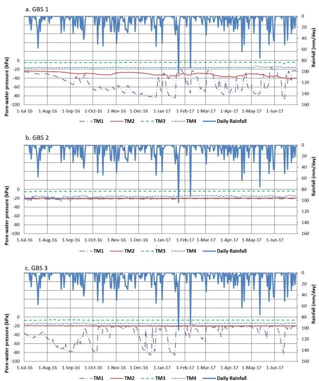
Figure 10. PWP recorded by Tensiometers in GBSs during monitoring period.
