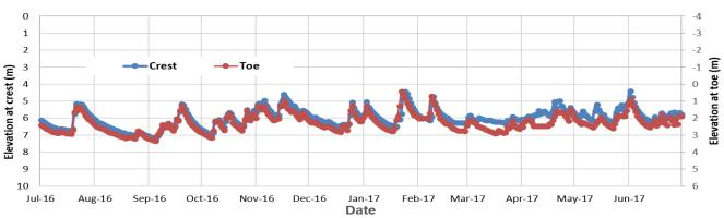
Figure 9. Groundwater table fluctuation in response to rainfall.
