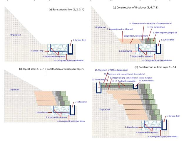
Figure 3. Construction stages of GBS.
