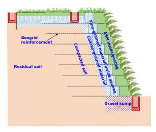
Figure 1. Schematic diagram of GBS.
