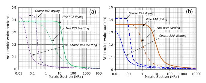
Figure 7. SWCCs of (a) fine RCA and coarse RCA and (b) fine RAP and coarse RAP.
