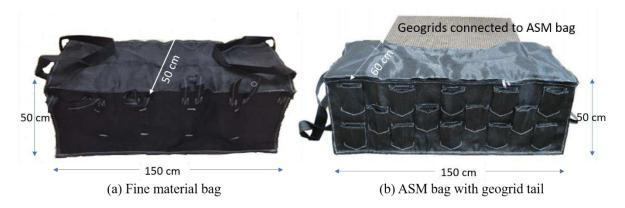
Figure 2. Geotextile bags for fine material and ASM.
