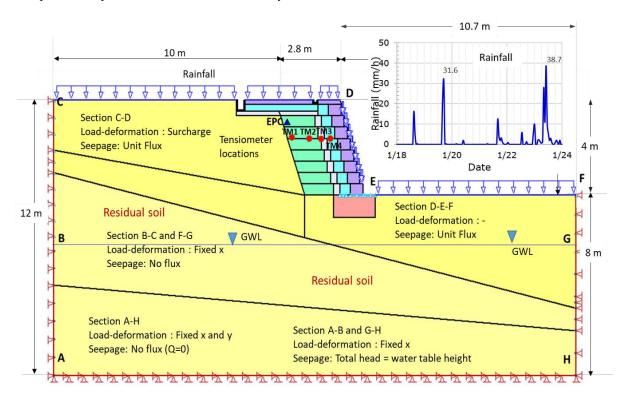
Figure 12. Finite element mesh and boundary conditions.
