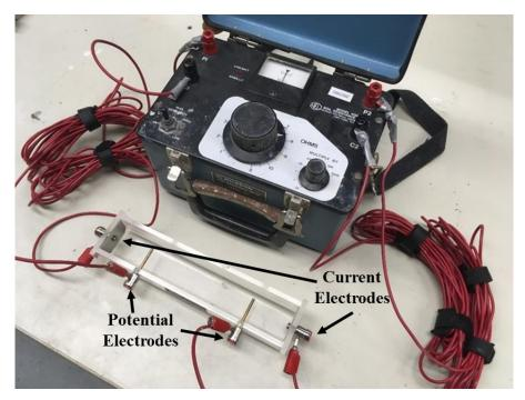
Figure 8. Laboratory resistivity setup.
