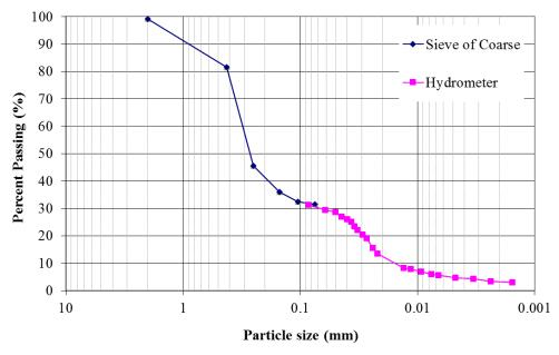
Figure 11. Particle size distribution for sample B1 retrieved from Sand Boil 1.
