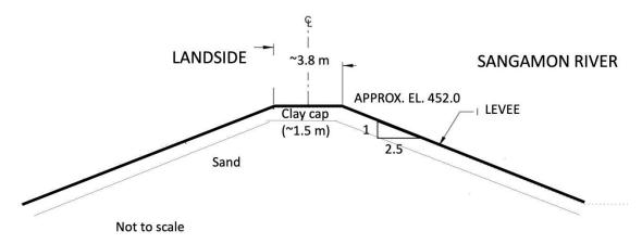
Figure 3. Hager Slough Levee pre-repair simplified cross-section.
