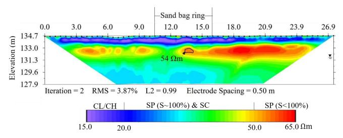
Figure 10. Line 3, survey near the landside toe that was 5.1 m uphill of sand bag ring.
