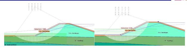
Figure 16 Left: View of scenario A. "Base model" using the Bishop slip circle and low values of POP resulting in FoS=0.69 (undrained soil behavior). Right: Scenario A. "Base model" using the Bishop model and low values of cohesion resulting in FoS=0.76 (drained soil behavior).
