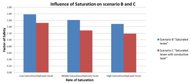
Figure 12. Blue: Influence of the saturation of the levee on the FoS. Red: Influence of the saturation when the local high water pressures in the conductive layer are introduced.
