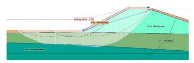
Figure 14 View of scenario D: "Pond connection with aquifer" output. The high hydraulic head is included and the Spencer model is used (with drained soil behavior) which results in FoS=1.42.
