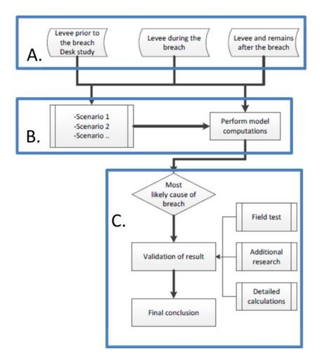
Figure 8. Generic approach for levee forensic analysis based on Borsje, et al. (2014) Step A.: Collecting information for exploring possible scenarios; Step B.: Evaluate with a computational model; Step C.: When results do not identify the cause, additional information can be gathered.
