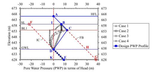
Figure 15. Maximum PWP profiles and PWP envelope for 500-year flood event at the SR-SCR bridge site.
