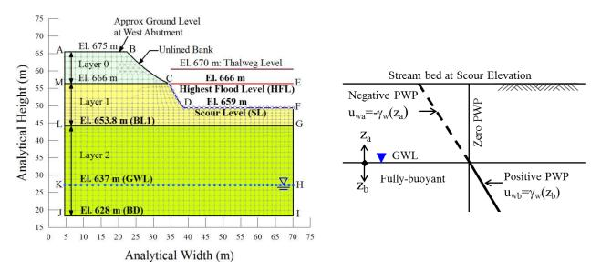
Figure 5. 2-D domain for infiltration analysis.
