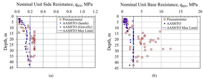
Figure 11. Profiles of Nominal Unit Resistance with Depth at 110-ItoR location for (a) Side, (b) Base.
