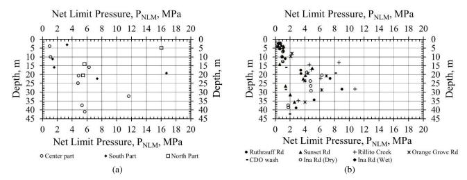
Figure 8.  $P_{NLM}$  Pressure profiles at (a) I10-I19 TI locations, (b) I10-ItoR locations.
