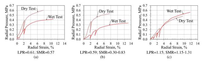
Figure 12. Dry and Wet Test Results at 110-Ina Road TI (a) Depth=2.3 m, (b) Depth=3.8 m, and (c) Depth=5.3 m.
