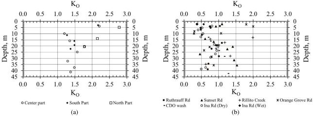
Figure 4. K<sub>O</sub> profiles at (a) I10-I19 TI locations, (b) I10-ItoR locations.
