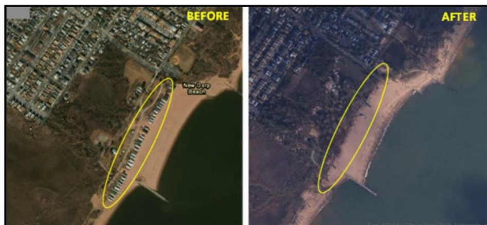
Figure 18. Aerial photographs from New Dorp Beach, SI, before and after Sandy. Row of houses completely removed and debris moved inland. (Images from tmappsevents.esri.com/website/swipe_sandy/ ).
