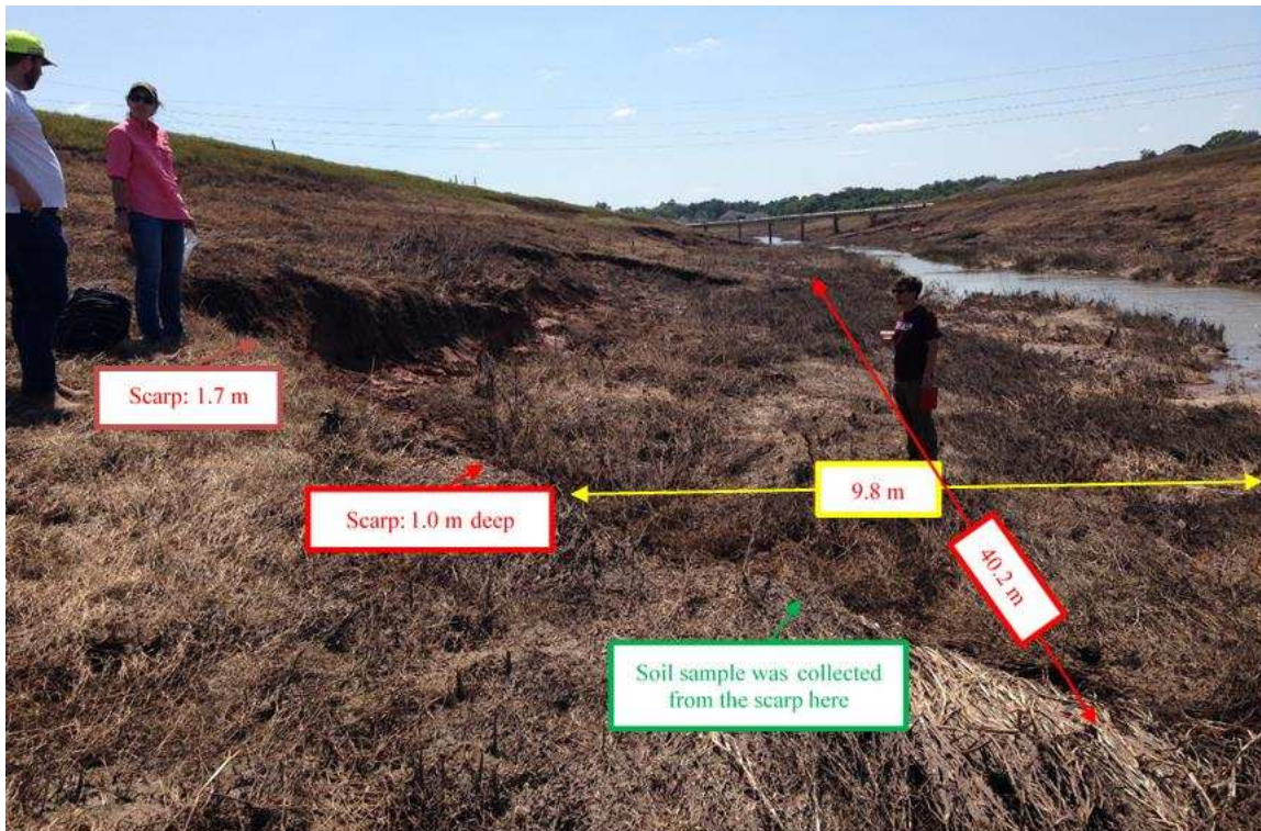
Figure 21. Slope failure north of damaged drainage pipe on the east side of ditch (September 10, 2017, 29.52647°N 95.56194°W),
