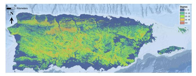
Figure 5. Slope map showing computed average slope inclinations from 5 m resolution DEM (Hughes and Morales-Velez, 2017; adapted from Silva-Tulla et al., 2018).
