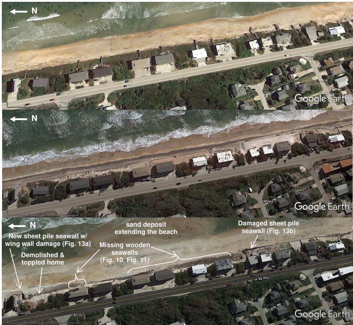
Figure 9: Changes to the Vilano Beach coastline from 4020 to 3880 Coastal Highway, St. Augustine, Florida, at 29^{\circ}56'49.30''N latitude and 81^{\circ}18'9.37''W longitude dated: (a) November 2015, with few seawalls present; (b) March 2017, with seawalls installed following 2016 Hurricane Matthew, and; (c) October 2018, following damage from 2017 Hurricane Irma (Google Earth, 2018).
