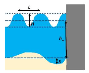
Figure 1. Schematic drawing of a vertical seawall (grey), seabed (beige), and water conditions (blue) introducing relevant symbols: scour depth in front of the seawall S, still water depth at the seawall S, wave length S, and wave height S.
