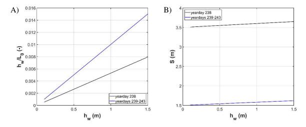
Figure 14. A) Water depth at the seawall  $h_w$  vs. the relationship between  $h_w$  and the deep water wave length  $L_0$  for conditions on yearday 238 (black) and yeardays 239-243 (blue). B) Estimated scour depths S within the same days and range of  $h_w$  after Equation 1 (Fowler 1992).
