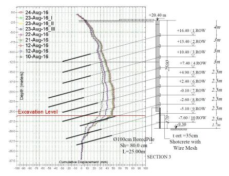
Figure 10. Encountered Excessive Displacements on Section 3.
