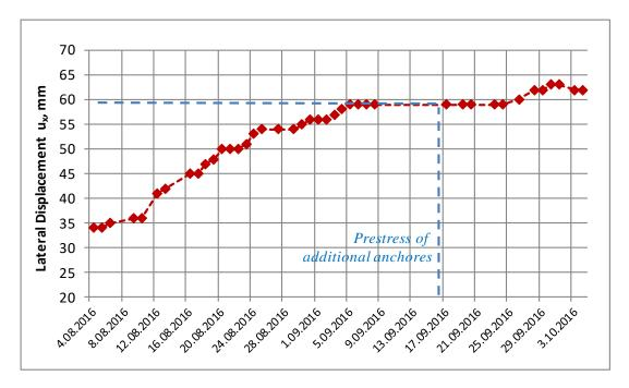
Figure 12. Section 3 Lateral Displacements.
