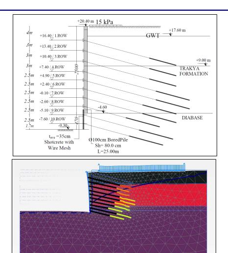
Figure 9. Section View of the Revised Retaining System.
