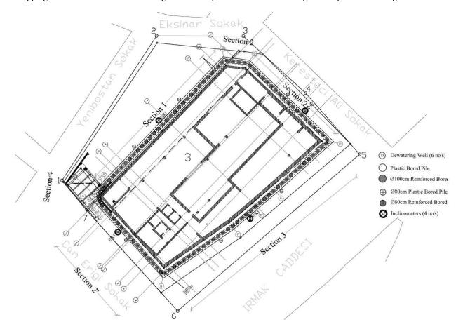
Figure 6. The Plan View of the Retaining System.
