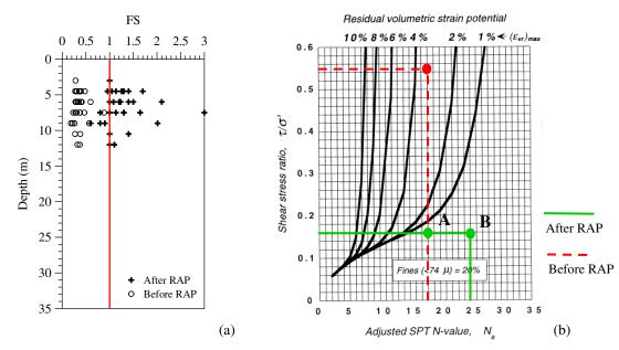
Figure 7. a) Liquefaction susceptibility of silty sand layer before and after RAP applications; b) Relationship between normalized SPT N value and shear strain potential for the case of FC=20 % (Shamoto et al., 1998).
