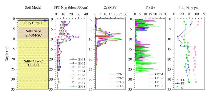
Figure 4. The representative soil profile, the variation of SPT N<sub>60</sub>, Q<sub>t</sub>, F<sub>r</sub>, LL, PI, and  $\Theta$  with depth.
