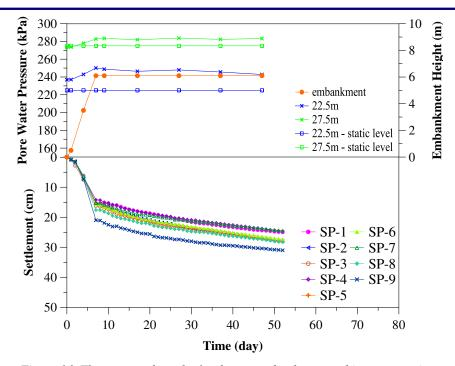
Figure 16. The measured results for the test embankment and instrumentation.
