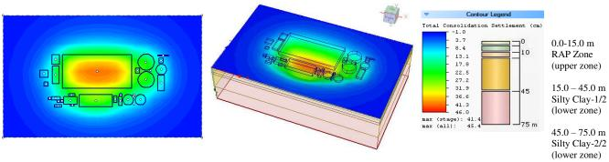
Figure 17. The consolidation settlements in the case of all structures constructed.
