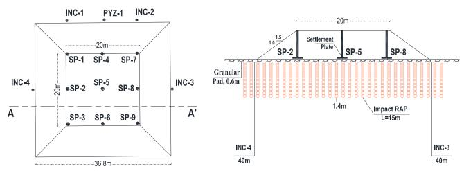
Figure 14. The layout plan and the section of test embankment.
