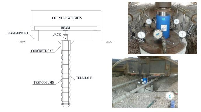
Figure 11. The test set-up and field photos.
