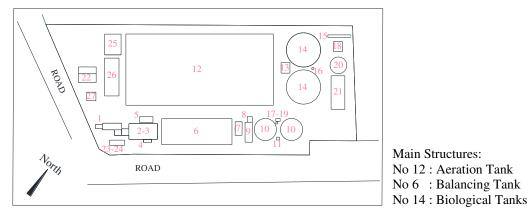
*Figure 2. The layout plan of wastewater treatment facility.*
