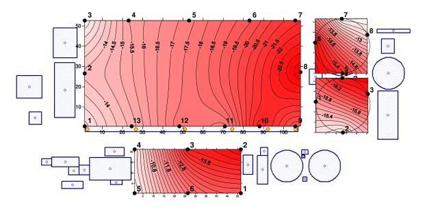
Figure 21. The distribution of measured final settlements on the plan.
