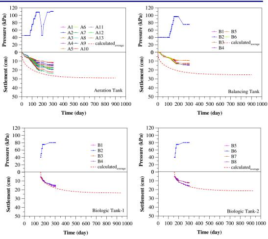
Figure 20. 3D model and field data responses: settlement vs. time curves for aeration, balancing, and biologic tanks.
