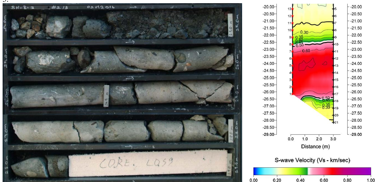
Figure 25. Core box photos of coring BH-B-3 between 24 and 29 m depth. Measured V_s across overlapping columns.
