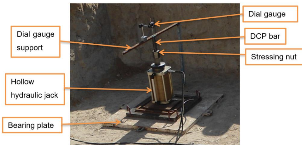
Figure 51. Typical arrangement of acceptance test.
