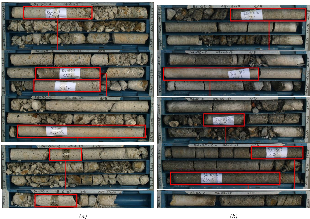
Figure 50. Core box photos of executed continuous coring: (a) QC-1 and (b) QC-2.
