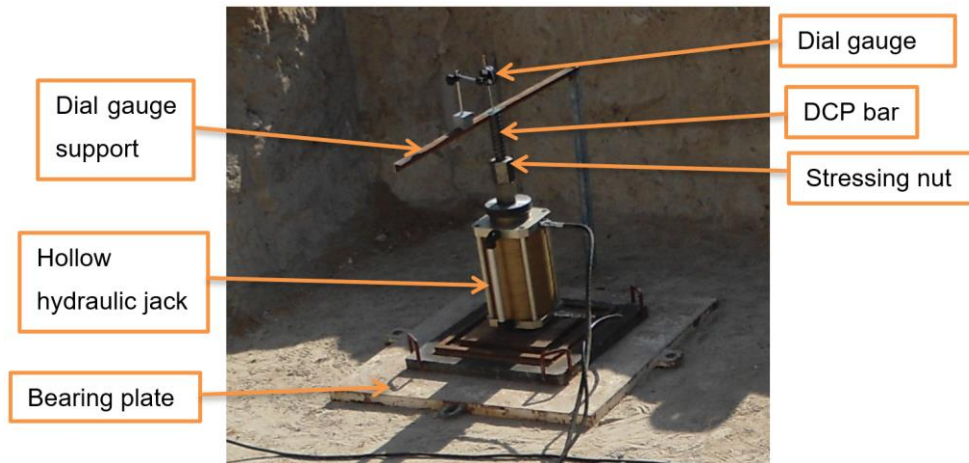
Figure 51. Typical arrangement of acceptance test.
