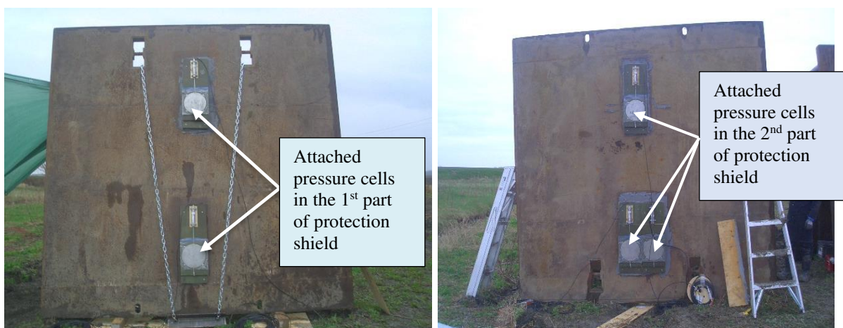
Figure 8. Pressure cells are fixed on the side of the first and second trench boxes.
