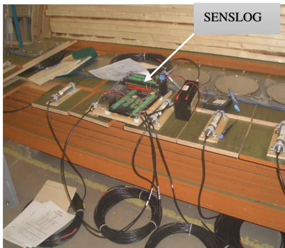
(c) Pressure cells were verified by the SENSLOG datalogger in the ETS lab before site installation.
