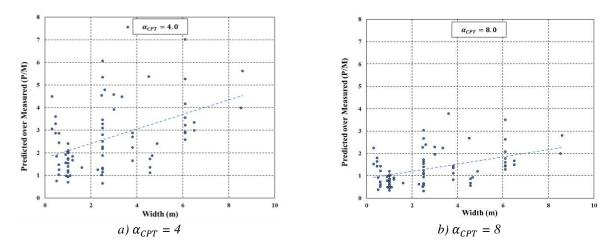
Figure 8. Predicted over measured settlement records versus width of foundation for TAMU-SHAL-SAND Database when using  $E(kPa) = 4 q_c(kPa)$  (90.4% of probability) and  $E(kPa) = 8 q_c(kPa)$  (54.6% of probability).
