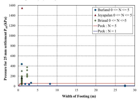
Figure 15. Comparison between pressures computed from three databases and Peck charts for  $0 \le N \le 5$ .
