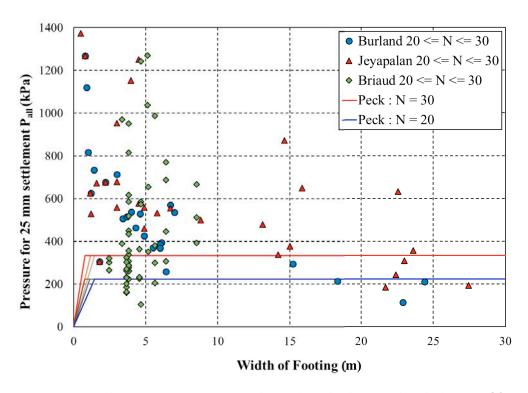
Figure 19. Comparison between pressures computed from three databases and Peck charts for  $20 \le N \le 30$ .
