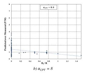
Figure 9. Predicted over measured settlement records versus depth of foundation over width of foundation  $(D_f/B)$  for TAMU-SHAL-SAND Database when using  $E(kPa) = 4 q_c(kPa)$  (90.4% of probability) and  $E(kPa) = 8 q_c(kPa)$  (54.6% of probability).
