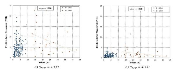
Figure 4. Predicted over measured settlement records versus width of foundation for TAMU-SHAL-SAND Database when using E(kPa) = 1000 N(91.2% of probability) and E(kPa) = 4000 N(49.3% of probability).
