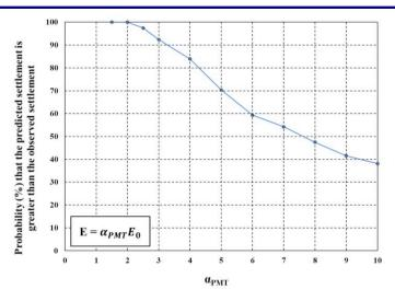
Figure 11. Probability plot based on PMT results for TAMU-SHAL-SAND Database.
