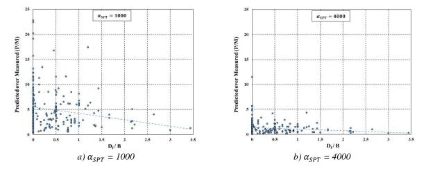
Figure 5. Predicted over measured settlement records versus depth over width of foundation ( $D_f/B$ ) for TAMU-SHAL-SAND Database when using E(kPa) = 1000 N(91.2% of probability) and E(kPa) = 4000 N(49.3% of probability).
