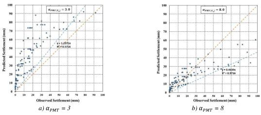
Figure 10. Predicted versus measured settlement records for TAMU-SHAL-SAND Database.
