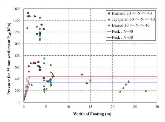
Figure 20. Comparison between pressures computed from three databases and Peck charts for  $30 \le N \le 40$ .
