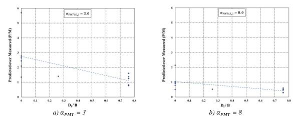
Figure 13. Predicted over measured settlement records versus depth of foundation over width of foundation  $(D_f/B)$  for TAMU-SHAL-SAND Database when using  $E(kPa) = 3 E_0(kPa)$  (92.3% of probability) and  $E(kPa) = 8 E_0(kPa)$  (47.5% of probability).
