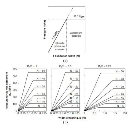
Figure 14. Peck chart providing the allowable bearing pressure for 25 mm settlement for footings on sand with SPT value (Terzaghi and Peck, 1963).
