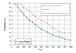
Figure 3. Probability of lower than predicted settlement occurence based on SPT results for all data in TAMU-SHAL-SAND Database, data with foundation widths smaller than 10 m, and data with foundation widths larger than 10 m.
