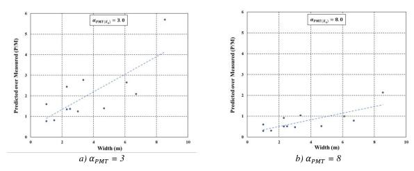
Figure 12. Predicted over measured settlement records versus width of foundation for TAMU-SHAL-SAND Database when using  $E(kPa) = 3 E_0(kPa)$  (92.3% of probability) and  $E(kPa) = 8 E_0(kPa)$  (47.5% of probability).
