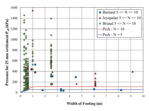
Figure 16. Comparison between pressures computed from three databases and Peck charts for  $5 \le N \le 10$ .
