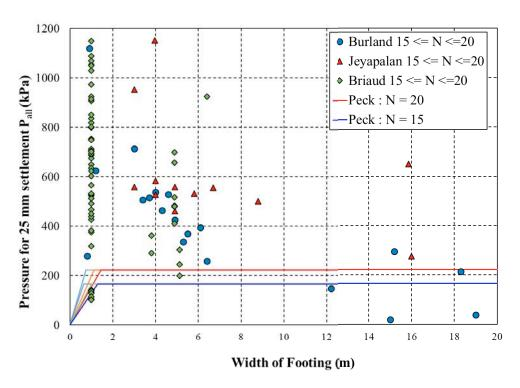
Figure 18. Comparison between pressures computed from three databases and Peck charts for  $15 \le N \le 20$ .
