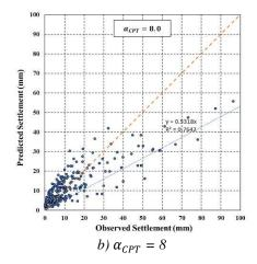
Figure 6. Predicted versus measured settlement records for TAMU-SHAL-SAND Database when using  $E(kPa) = 4 q_c(kPa)$ .
