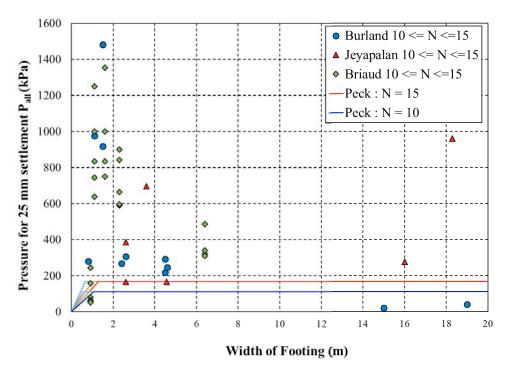
Figure 17. Comparison between pressures computed from three databases and Peck charts for  $10 \le N \le 15$ .
